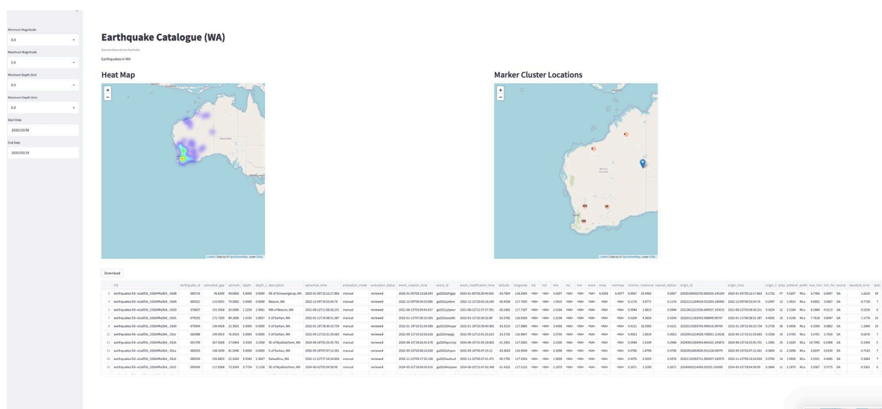
Figure 1 Screenshot of the Streamlit-based interface showing the earthquake heat map (left) and cluster map (right). The heat map highlights areas with high concentrations of detected events, while the cluster map groups closely spaced events for easier visualisation. The lower panel of the interface displays a searchable, filterable event catalogue . Users can download the catalogue and apply custom filters based on time, magnitude, and depth.
