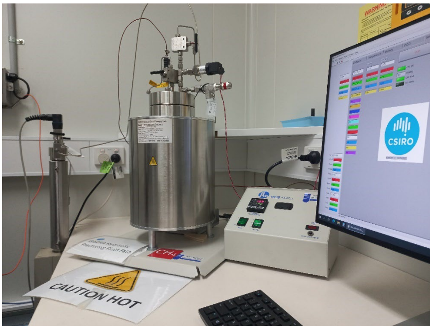
Figure 3: High pressure and temperature batch reactor rig with one cell at CSIRO Clayton laboratory
