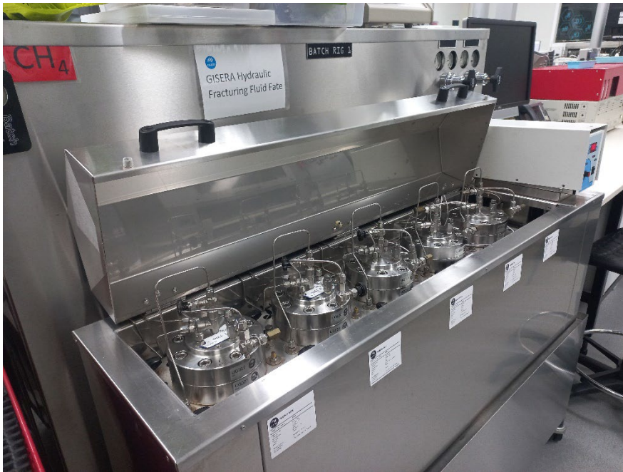
Figure 2: Batch reactor rig with 5 cells at the CSIRO Clayton laboratory
