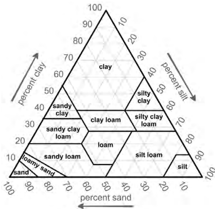
Figure 8 USDA Soil texture triangle
