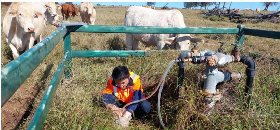
Taking water samples from an agricultural bore in the Surat Basin.
