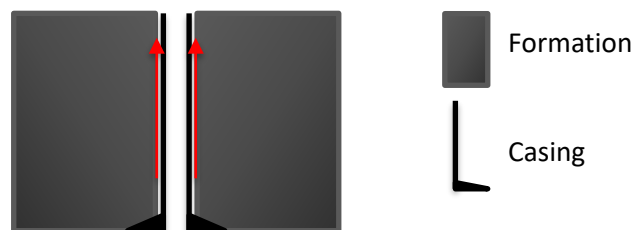
Figure 64: Potential leakage pathways at the interface of the casing and the rock formation (annulus)
