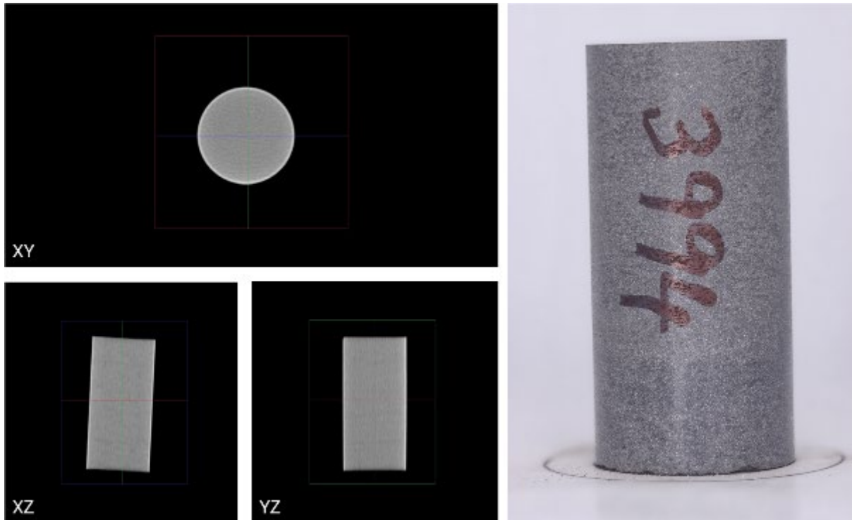
Figure 33: Axial and longitudinal XRCT 2D slices (a) and a picture of sample 3994 before sodium silicate solution saturation and creep MSTXL testing (b)
