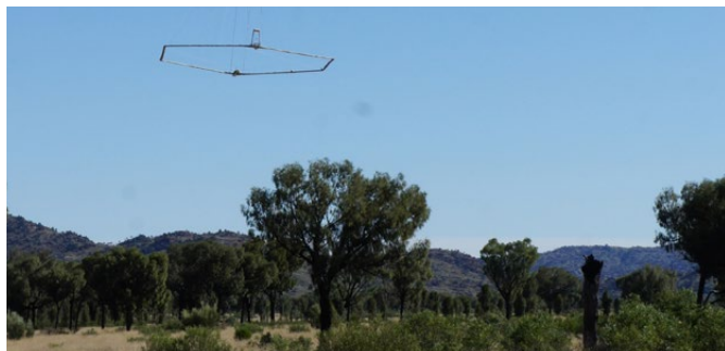
The carbon-fibre frame being towed by the helicopter emits a weak electromagnetic signal that detects changes in sub-surface conditions.
