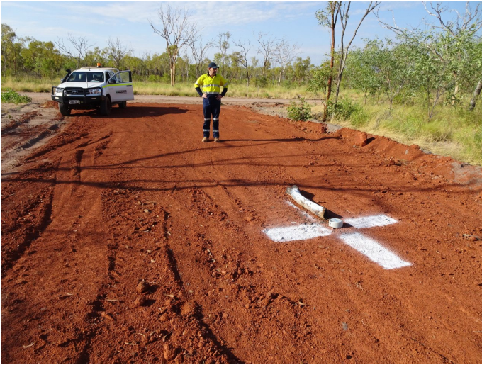
Figure 3 Example of ground control point. Eight were established across the property prior to aerial photography. Post Processing Kinematic (PPK) units (see photograph) were used at each ground control point to correct location data.
