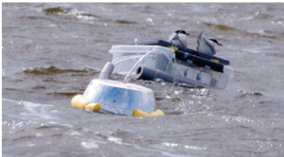
Figure 7 Example of an automated floating chamber (Reprinted with permission from Duc et al 2013, Copyright ©(2013), American Geophysical Union)
