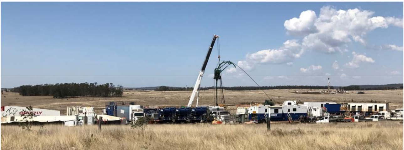
Figure 10: A hydraulic fracturing spread in the Roma-Yuleba region of the Surat Basin
