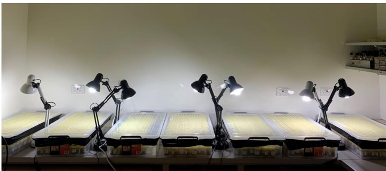
Figure 12: Microcosm incubation (with loose lids) stored in polypropylene containers with open vessels of a saturated salt (NaBr) for humidity control.
