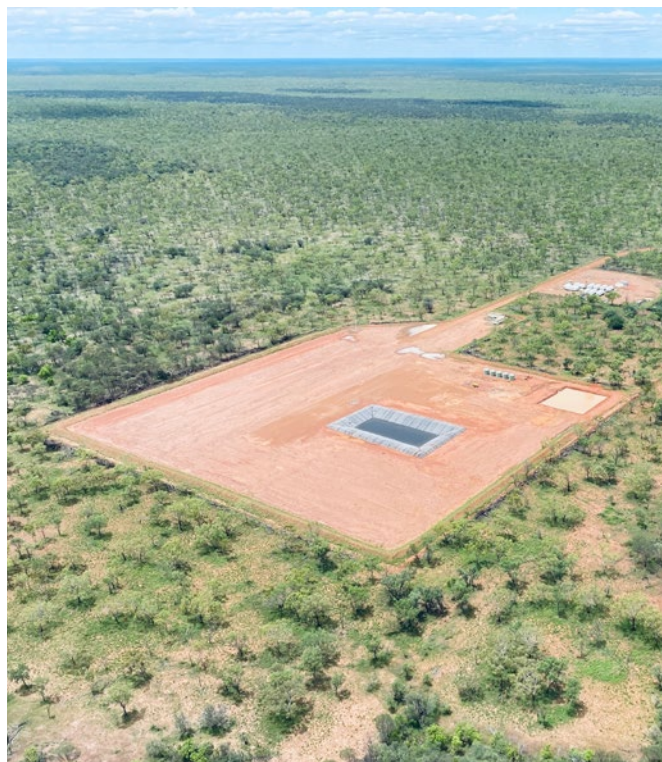
An exploration well pad in the Beetaloo Sub-basin, Northern Territory.
