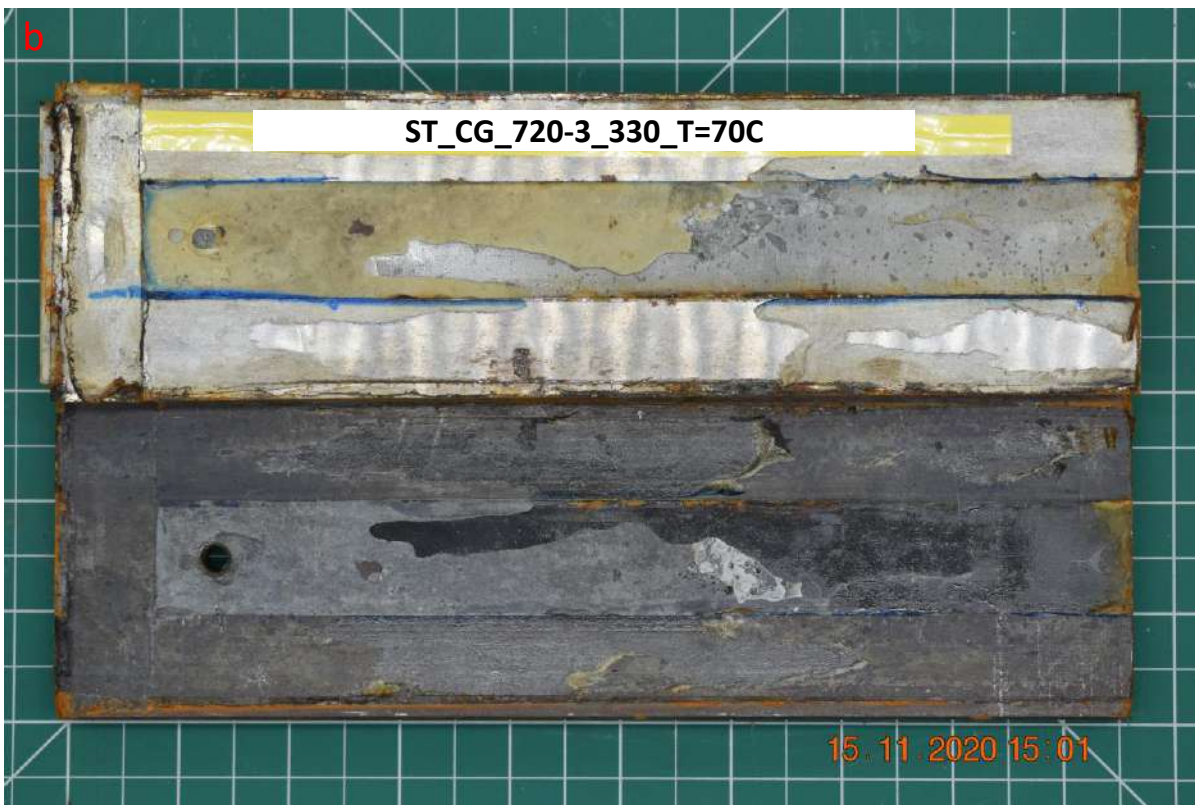
Figure C. 36. Injection test for fracture sample ST_CG_720-3_330_T=70C, a) Injection pressure, rate, force and volume vs time, and b) Photo of tested sample.
