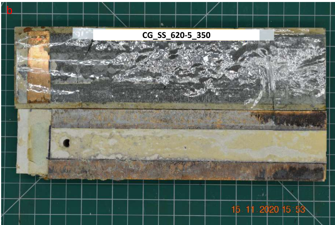
Figure C. 21. Injection test for fracture sample CG_SS_620-5_350, a) Injection pressure, rate, force and volume vs time, and b) Photo of tested sample following shear bonding strength test.
