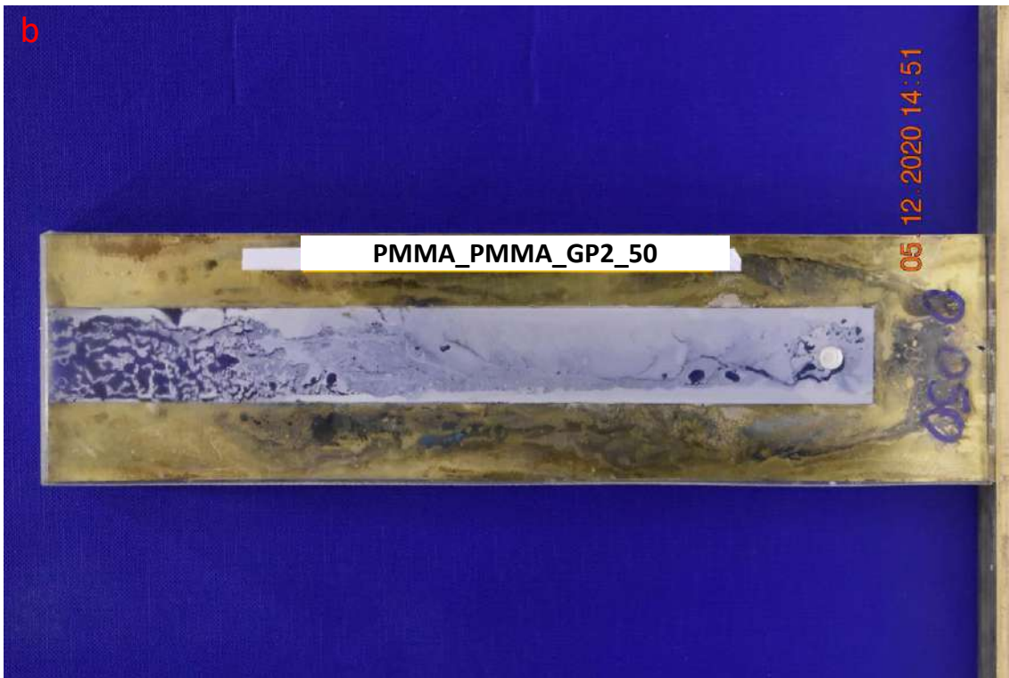
Figure C. 13. Injection test for fracture sample PMMA_PMMA_GP2_50, a) Injection pressure, rate, force and volume vs time, and b) Photo of tested sample.
