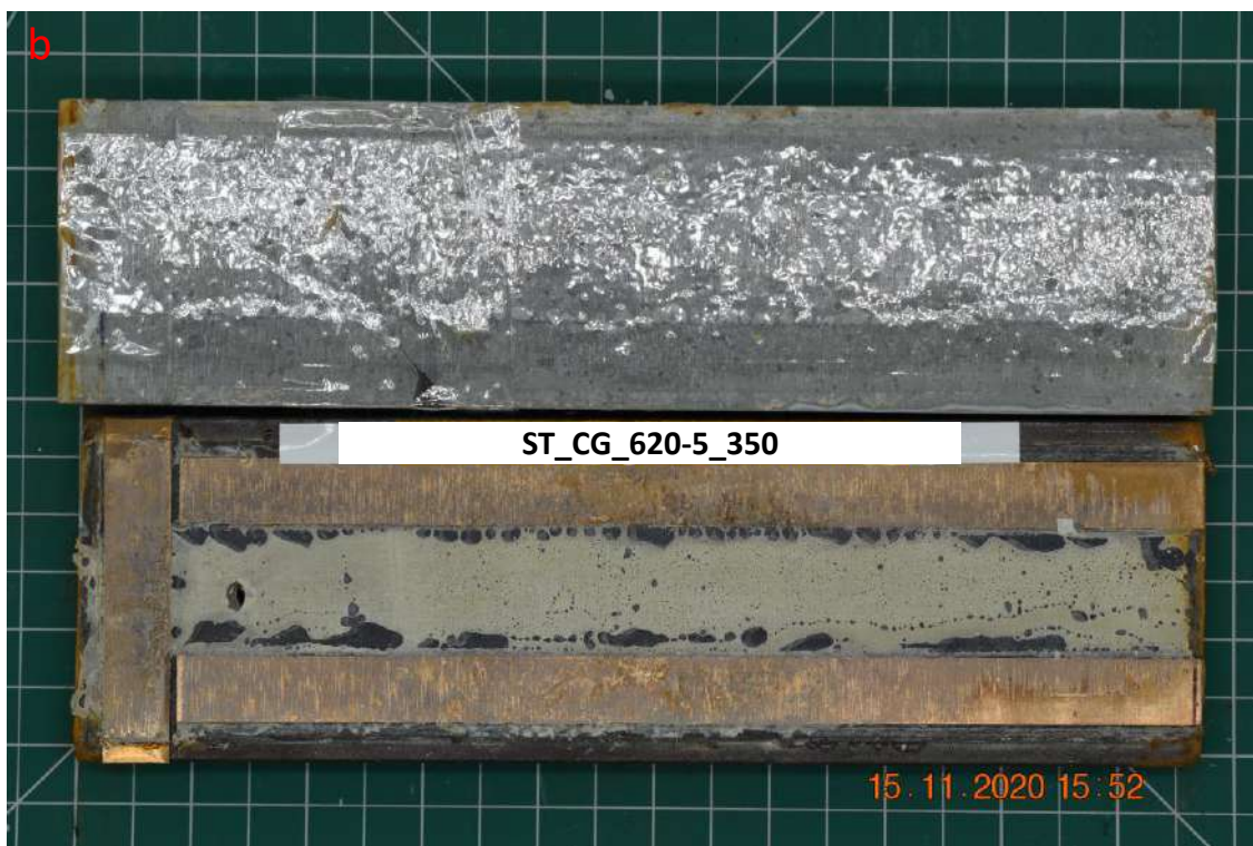
Figure C. 20. Injection test for fracture sample ST_CG_620-5_350, a) Injection pressure, rate, force and volume vs time, and b) Photo of tested sample after shear bonding strength test.
