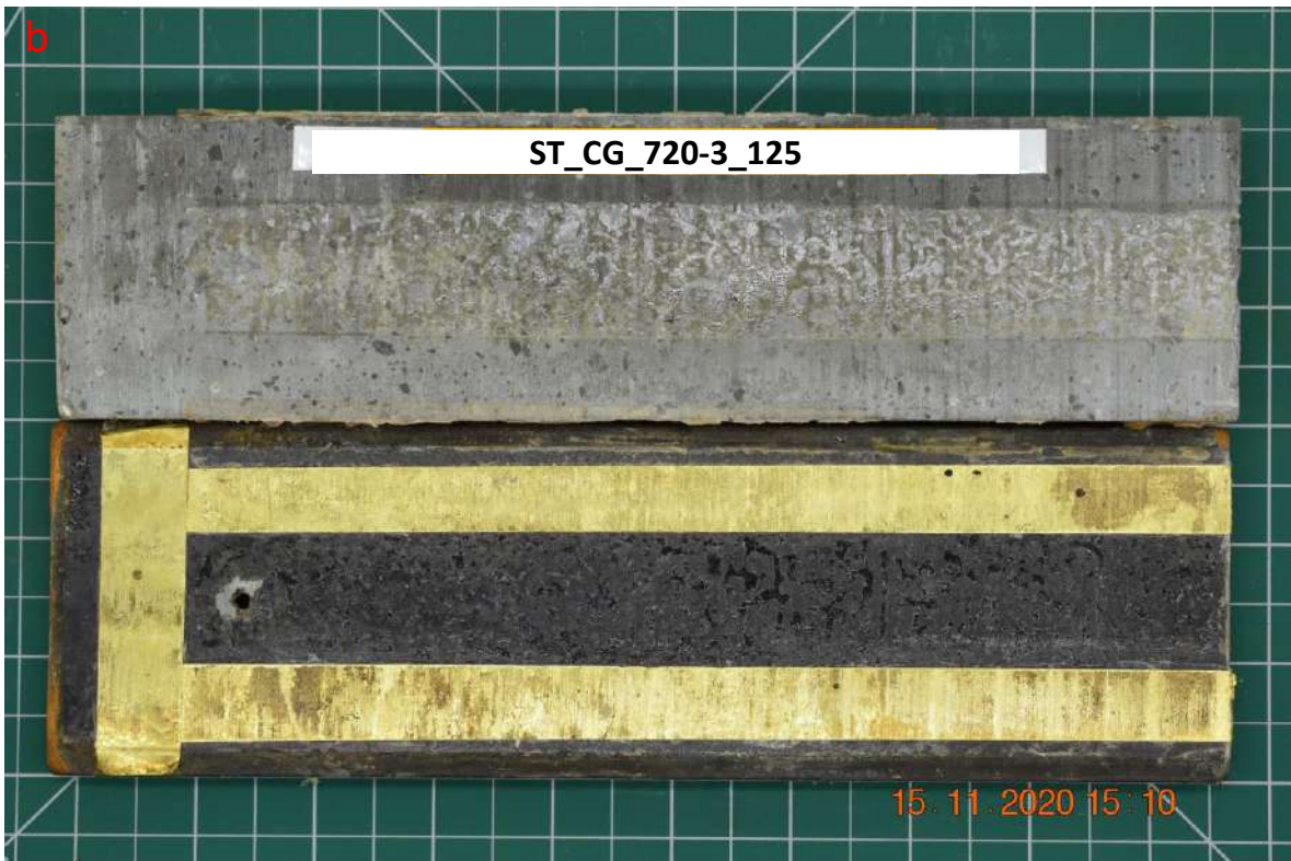
Figure C. 33. Injection test for fracture sample ST_CG_720-3_125, a) Injection pressure, rate, force and volume vs time, and b) Photo of tested sample.
