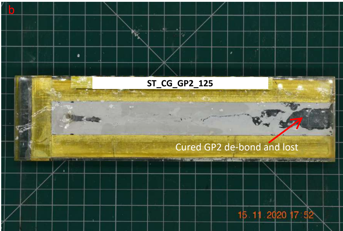
Figure C. 12. Injection test for fracture sample PMMA_PMMA_GP2_125, a) Injection pressure, rate, force and volume vs time, and b) Photo of tested sample.
