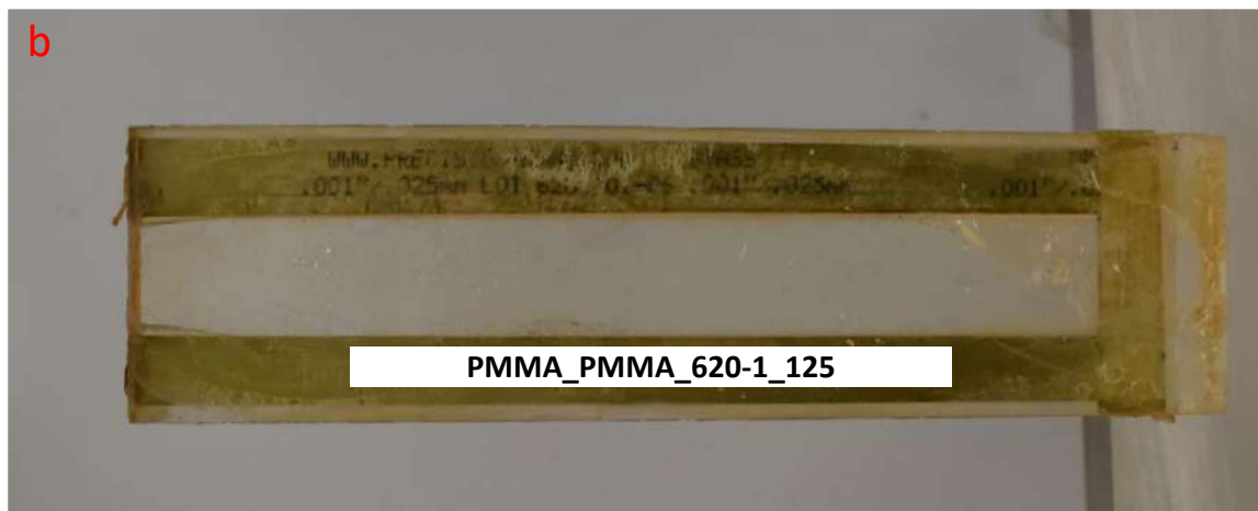
Figure C. 19. Injection test for fracture sample PMMA_PMMA_620-1_125, a) Injection pressure, rate, force and volume vs time, and b) Photo of tested sample.
