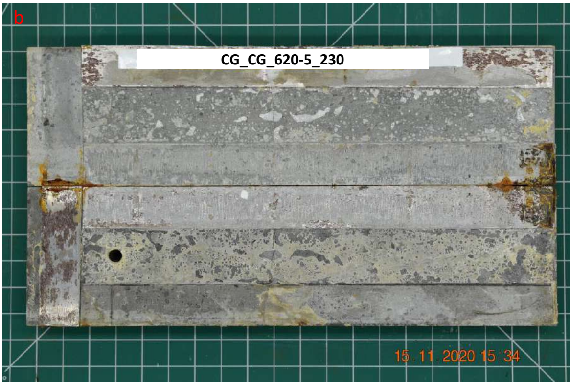
Figure C. 23. Injection test for fracture sample CG_ CG_620-5_230, a) Injection pressure, rate, force and volume vs time, and b) Photo of tested sample.
