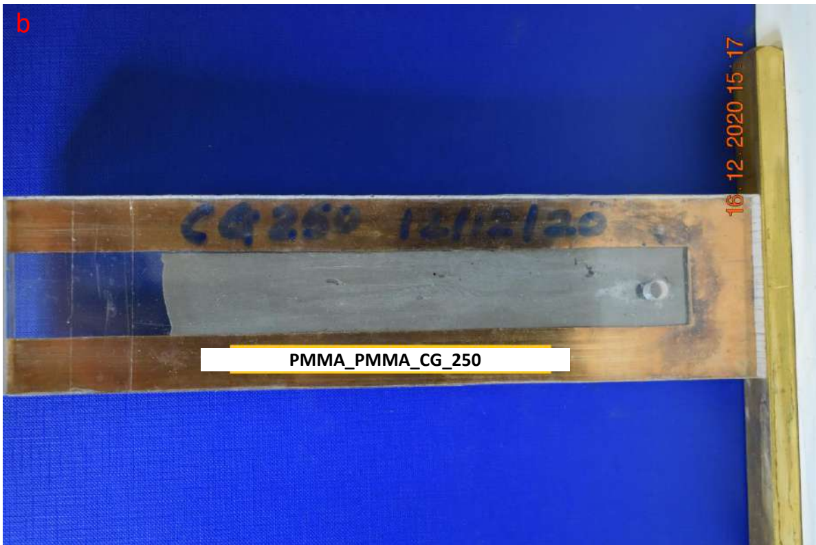
Figure C. 5. Injection test for fracture sample PMMA_PMMA_CG_250, a) Injection pressure, rate, force and volume vs time, and b) Photo of tested sample.
