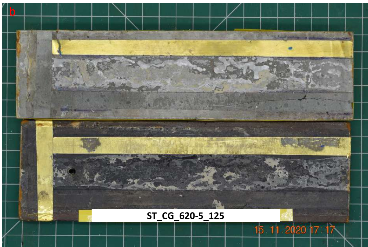
Figure C. 25. Injection test for fracture sample ST_CG_620-5_125, a) Injection pressure, rate, force and volume vs time, and b) Photo of tested sample.
