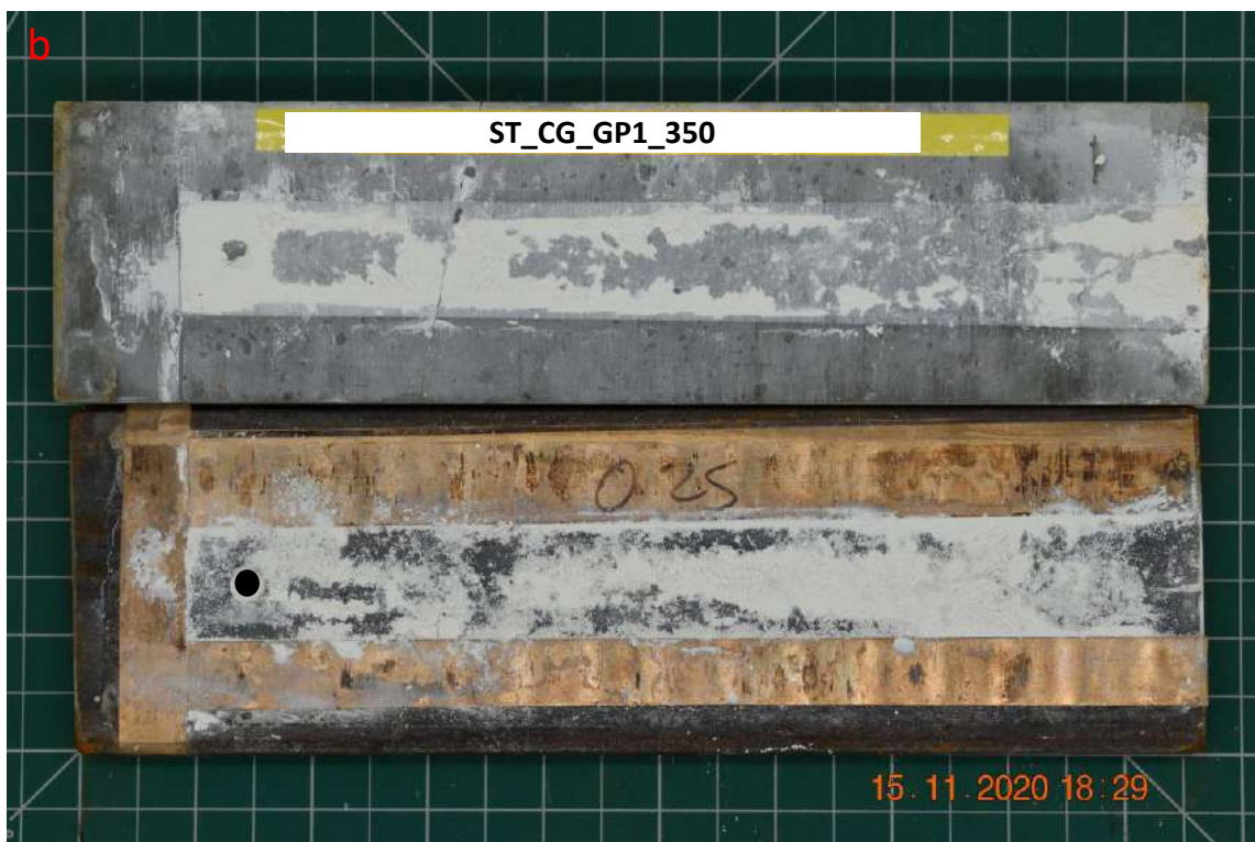
Figure C. 6. Injection test for fracture sample ST_CG_GP1_350, a) Injection pressure, rate, force and volume vs time, and b) Photo of tested sample after shear bonding strength test.
