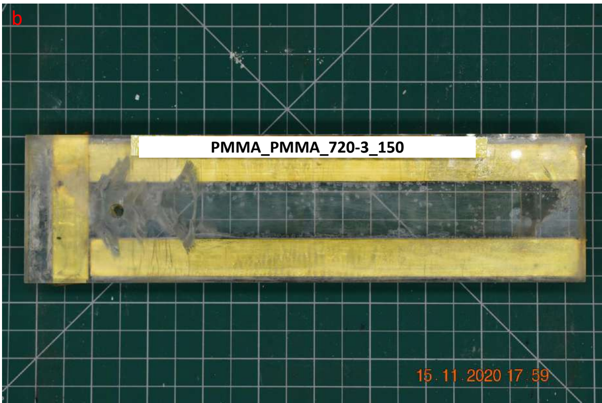
Figure C. 38. Injection test for fracture sample PMMA_PMMA_720-3_150, a) Injection pressure, rate, force and volume vs time, and b) Photo of tested sample. Shear bonding strength testing resulted in cracks in PMMA, not along the fracture.
