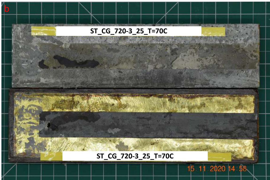
Figure C. 28. Injection test for fracture sample ST_CG_720-3_25_T=70C, a) Injection pressure, rate, force and volume vs time, and b) Photo of tested sample after shear bonding strength test.
