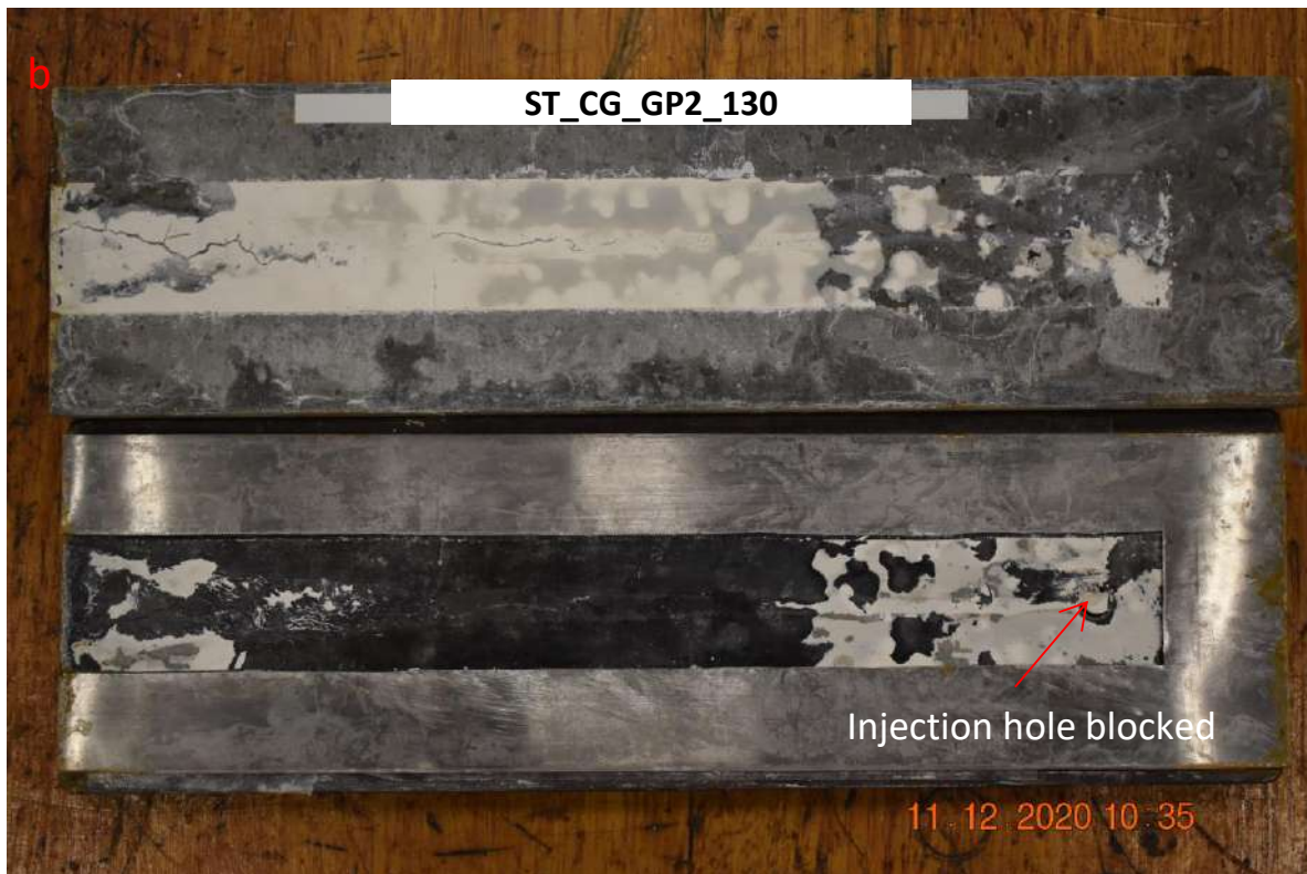
Figure C. 10. Injection test for fracture sample ST_CG_GP2_130, a) Injection pressure, rate, force and volume vs time, and b) Photo of tested sample after shear bonding strength test.
