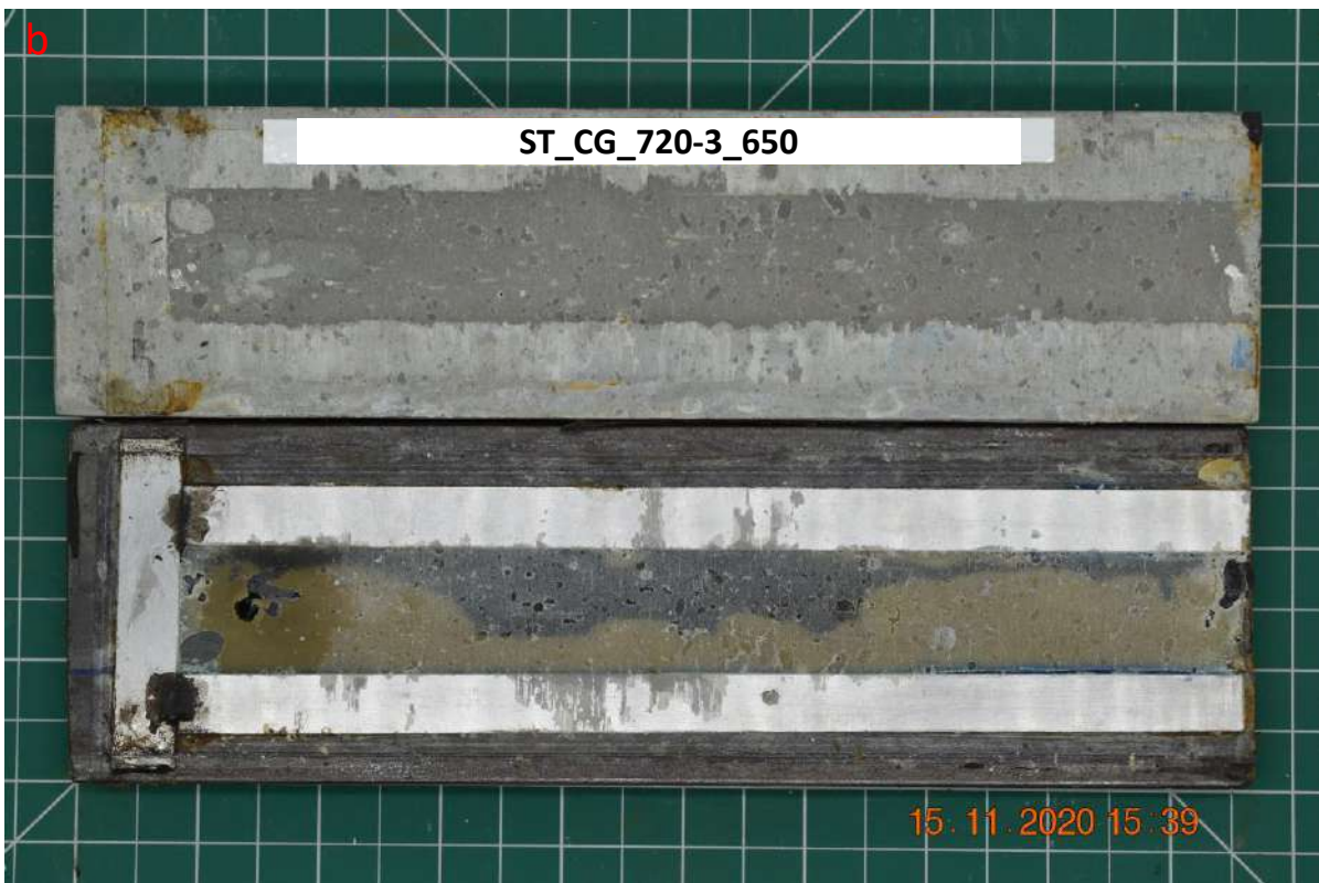
Figure C. 37. Injection test for fracture sample ST_CG_720-3_650, a) Injection pressure, rate, force and volume vs time, and b) Photo of tested sample.
