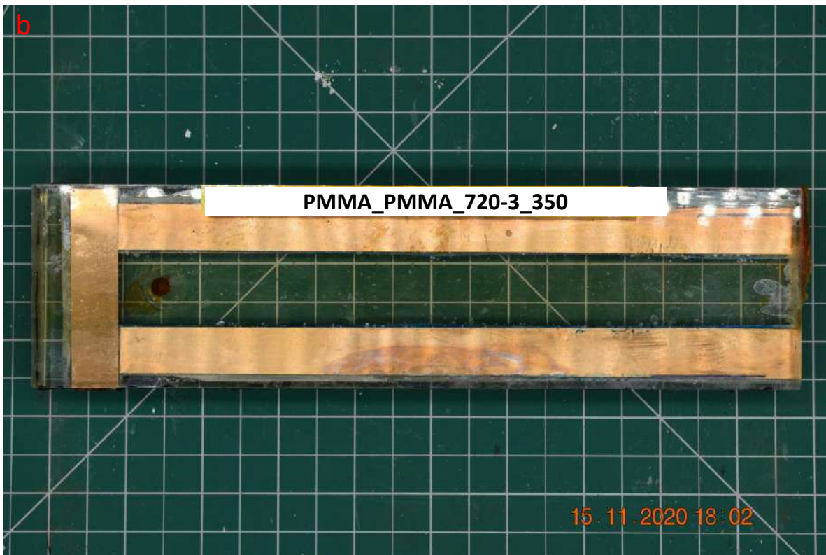
Figure C. 39. Injection test for fracture sample PMMA_PMMA_720-3_350, a) Injection pressure, rate, force and volume vs time, and b) Photo of tested sample. No shear bonding strength test.
