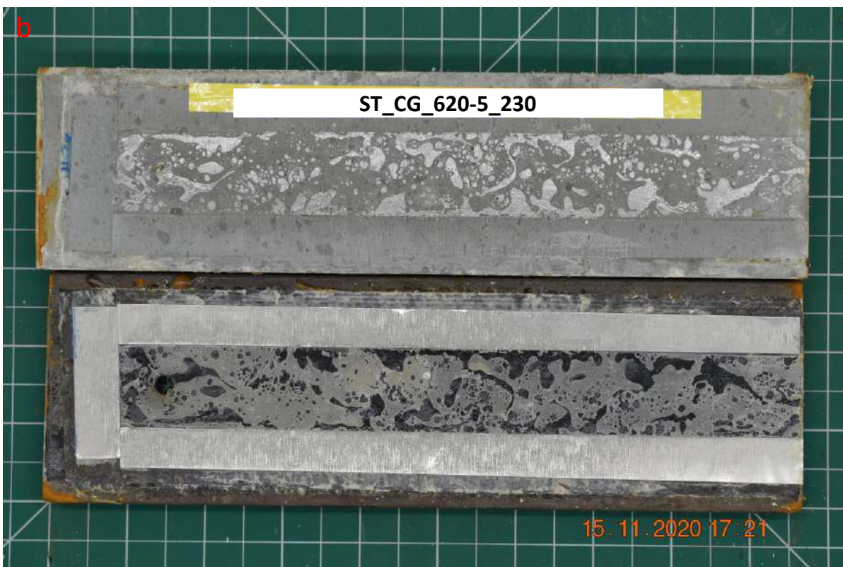
Figure C. 22. Injection test for fracture sample ST_CG_620-5_230, a) Injection pressure, rate, force and volume vs time, and b) Photo of tested sample after shear bonding strength test.
