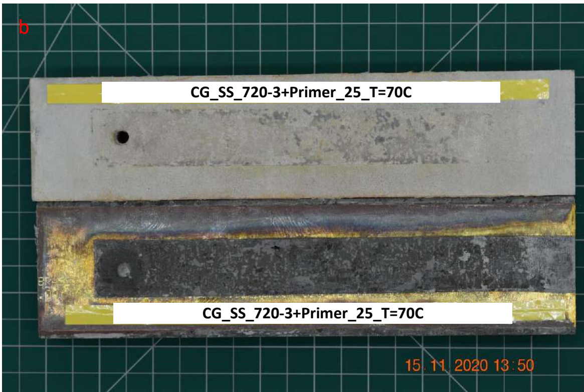
Figure C. 32. Injection test for fracture sample CG_SS_720-3+Primer_25_T=70C, a) Injection pressure, rate, force and volume vs time, and b) Photo of tested sample.
