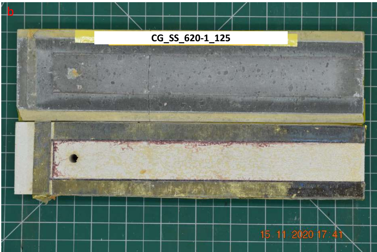
Figure C. 18. Injection test for fracture sample CG_SS_620-1_125, a) Injection pressure, rate, force and volume vs time, and b) Photo of tested sample.
