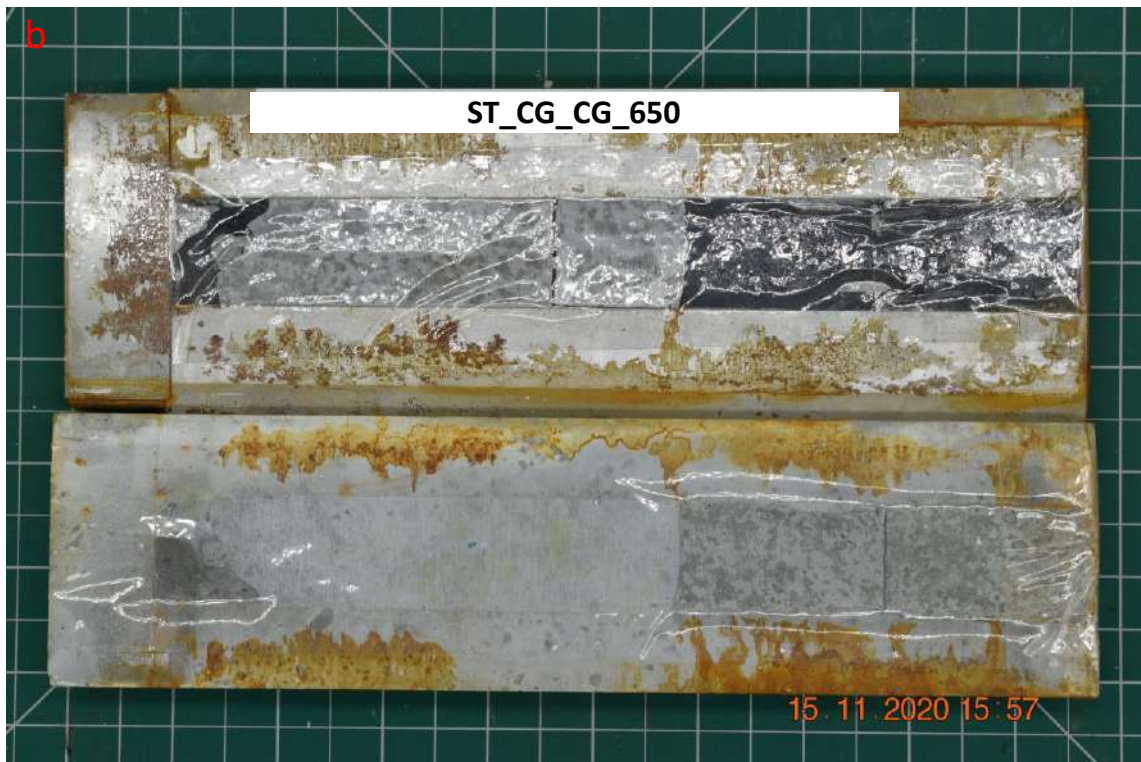
Figure C. 1. Injection test for fracture sample ST_CG_CG_650, a) Injection pressure, rate, force and volume vs time, and b) Photo of tested sample after shear bonding strength test.
