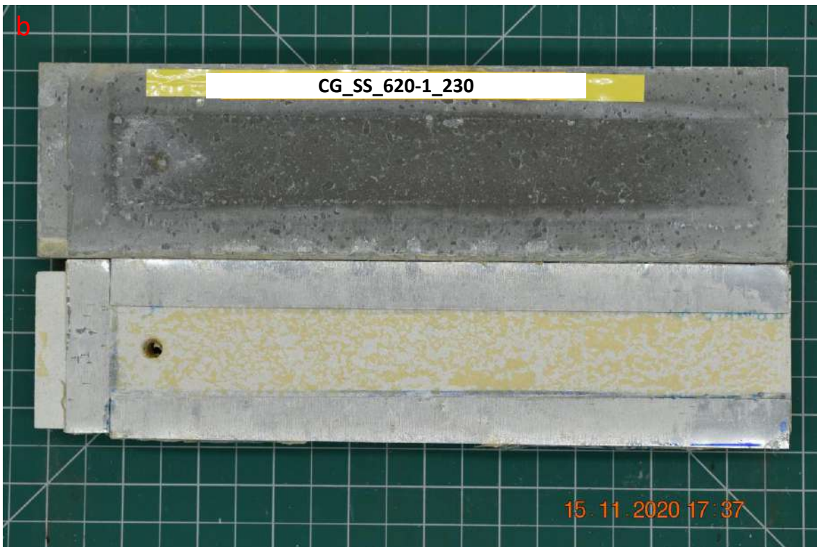
Figure C. 16. Injection test for fracture sample CG_SS_620-1_230, a) Injection pressure, rate, force and volume vs time, and b) Photo of tested sample following shear bonding strength test.
