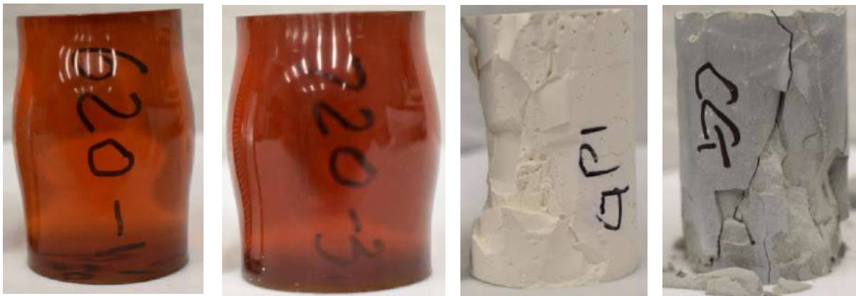
Figure B. 4. Photos of the tested samples for polymer resins, geopolymer and Class G cement, showing ductile deformation for polymer resin and brittle failure for geopolymer and Class G cement.
