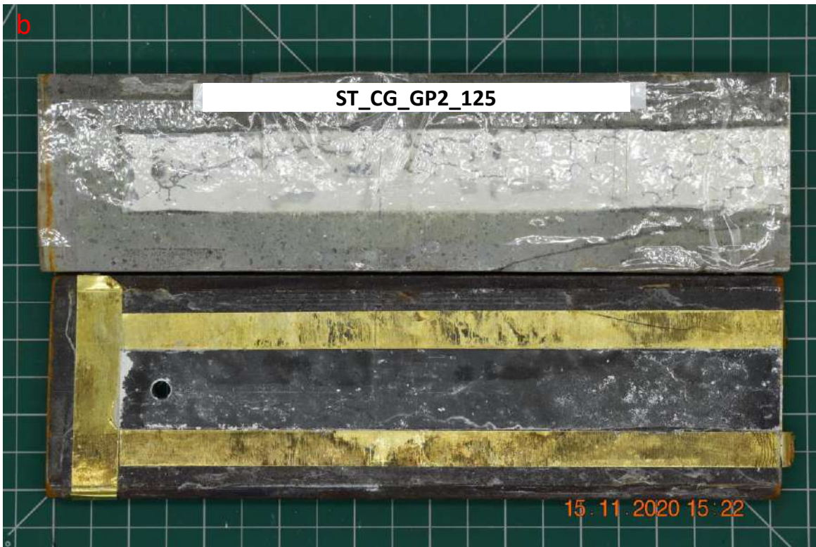
Figure C. 11. Injection test for fracture sample ST_CG_GP2_125, a) Injection pressure, rate, force and volume vs time, and b) Photo of tested sample following shear bonding strength test.
