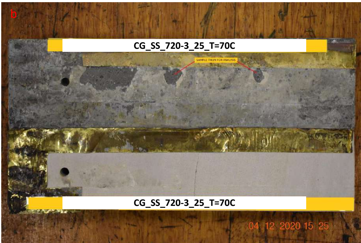
Figure C. 31. Injection test for fracture sample CG_SS_720-3_25_T=70C, a) Injection pressure, rate, force and volume vs time, and b) Photo of tested sample.
