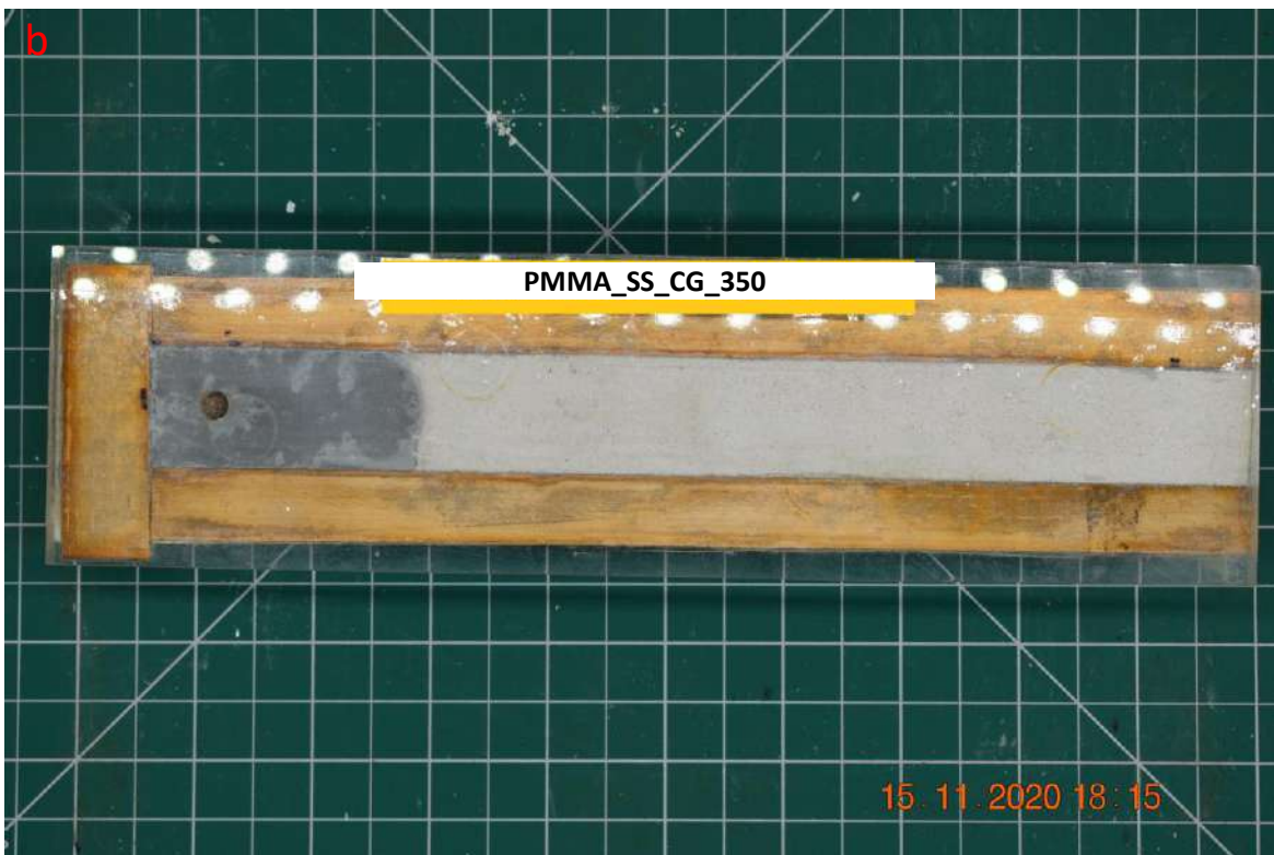
Figure C. 3. Injection test for fracture sample PMMA_SS_CG_350, a) Injection pressure, rate, force and volume vs time, and b) Photo of tested sample.
