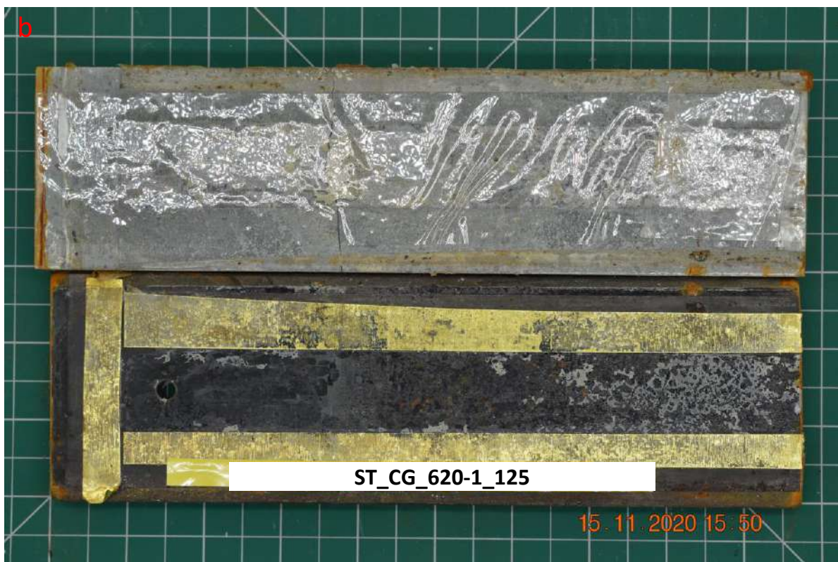
Figure C. 17. Injection test for fracture sample ST_CG_620-1_125, a) Injection pressure, rate, force and volume vs time, and b) Photo of tested sample. Note a layer of plastic tape covered the fracture surface to hold the cement slab together, which was broken following the shear bonding test.
