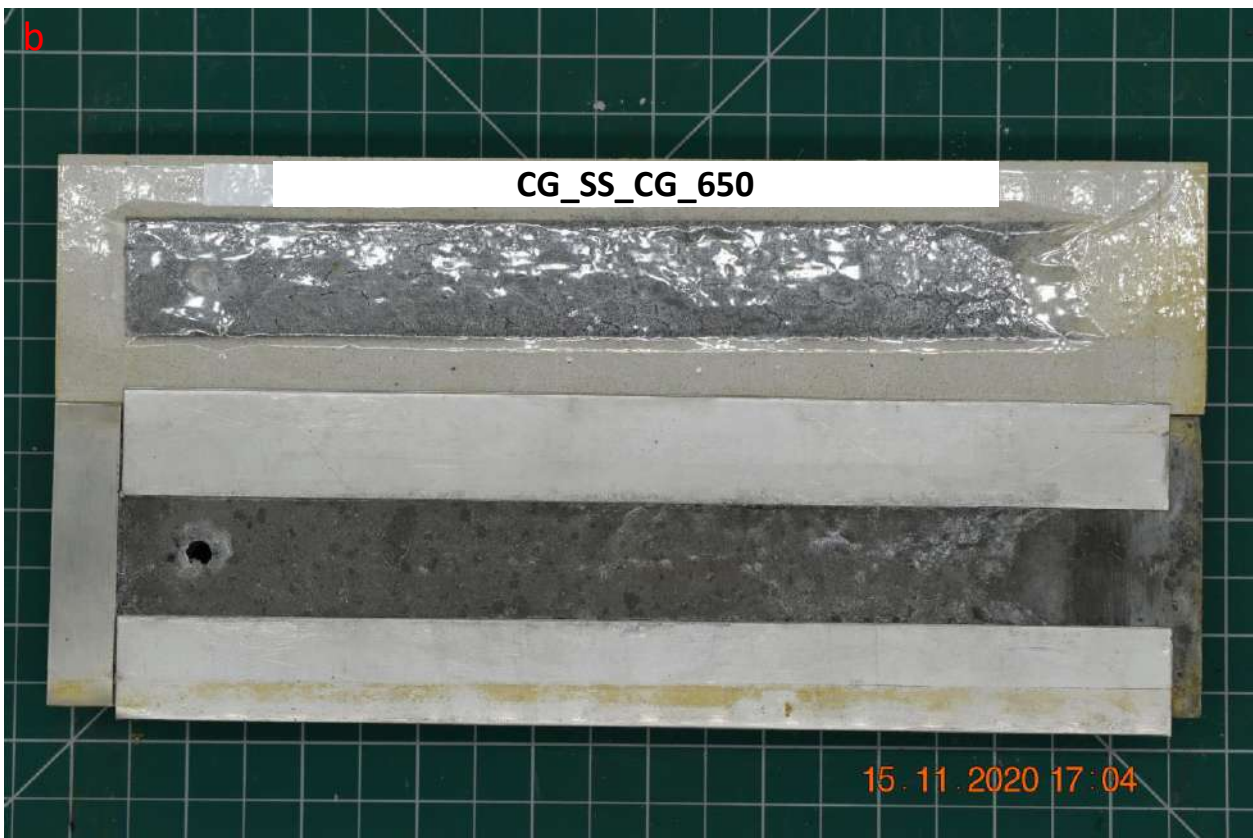
Figure C. 2. Injection test for fracture sample CG_SS_CG_650, a) Injection pressure, rate, force and volume vs time, and b) Photo of tested sample following shear bonding strength test.
