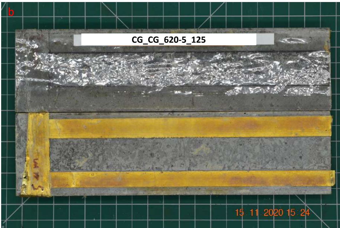
Figure C. 26. Injection test for fracture sample CG_620-5_125, a) Injection pressure, rate, force and volume vs time, and b) Photo of tested sample.
