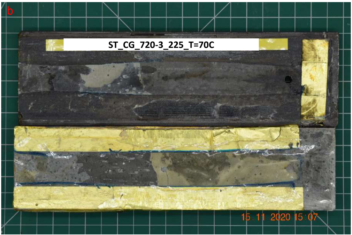
Figure C. 35. Injection test for fracture sample ST_CG_720-3_225_T=70C, a) Injection pressure, rate, force and volume vs time, and b) Photo of tested sample.
