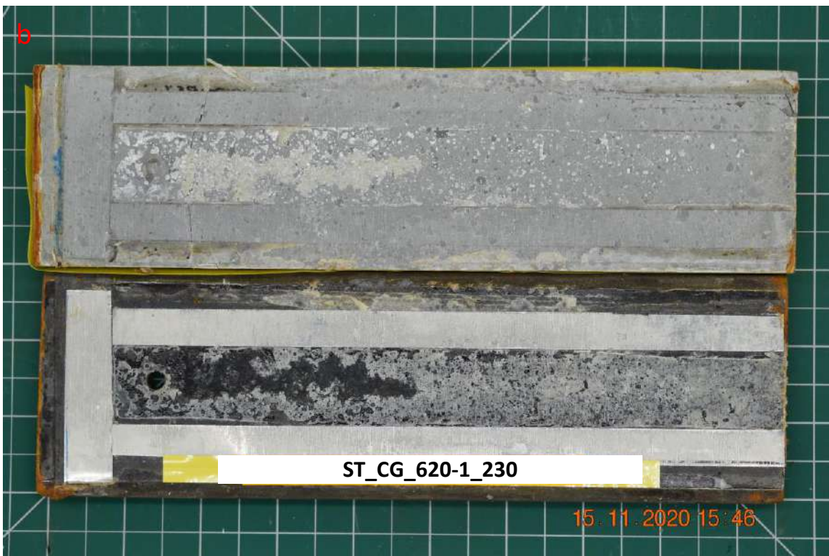
Figure C. 15. Injection test for fracture sample ST_CG_GP_620-1_230, a) Injection pressure, rate, force and volume vs time, and b) Photo of tested sample after shear bonding strength test.
