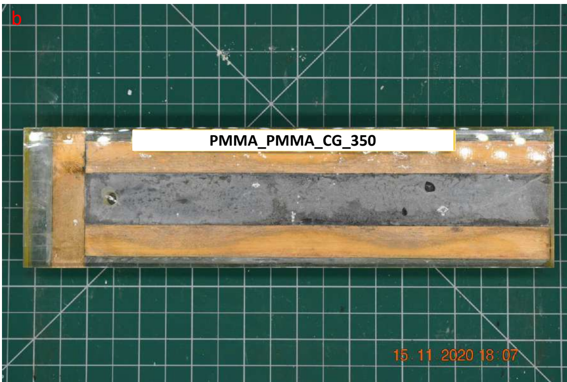
Figure C. 4. Injection test for fracture sample PMMA_PMMA_CG_350, a) Injection pressure, rate, force and volume vs time, and b) Photo of tested sample.
