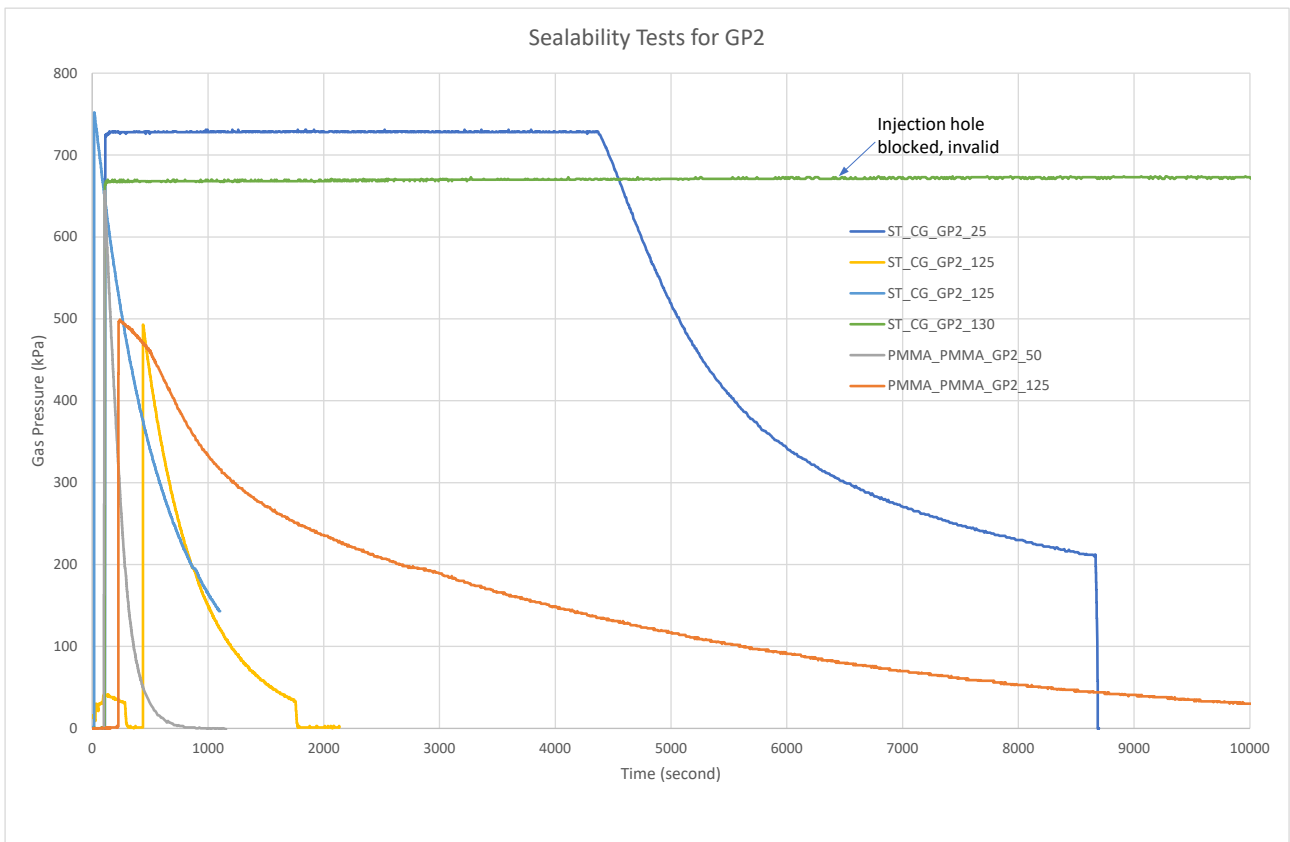
Figure 4-4. Gas pressure vs time for planar fractures sealed with geopolymer 2 slurries
