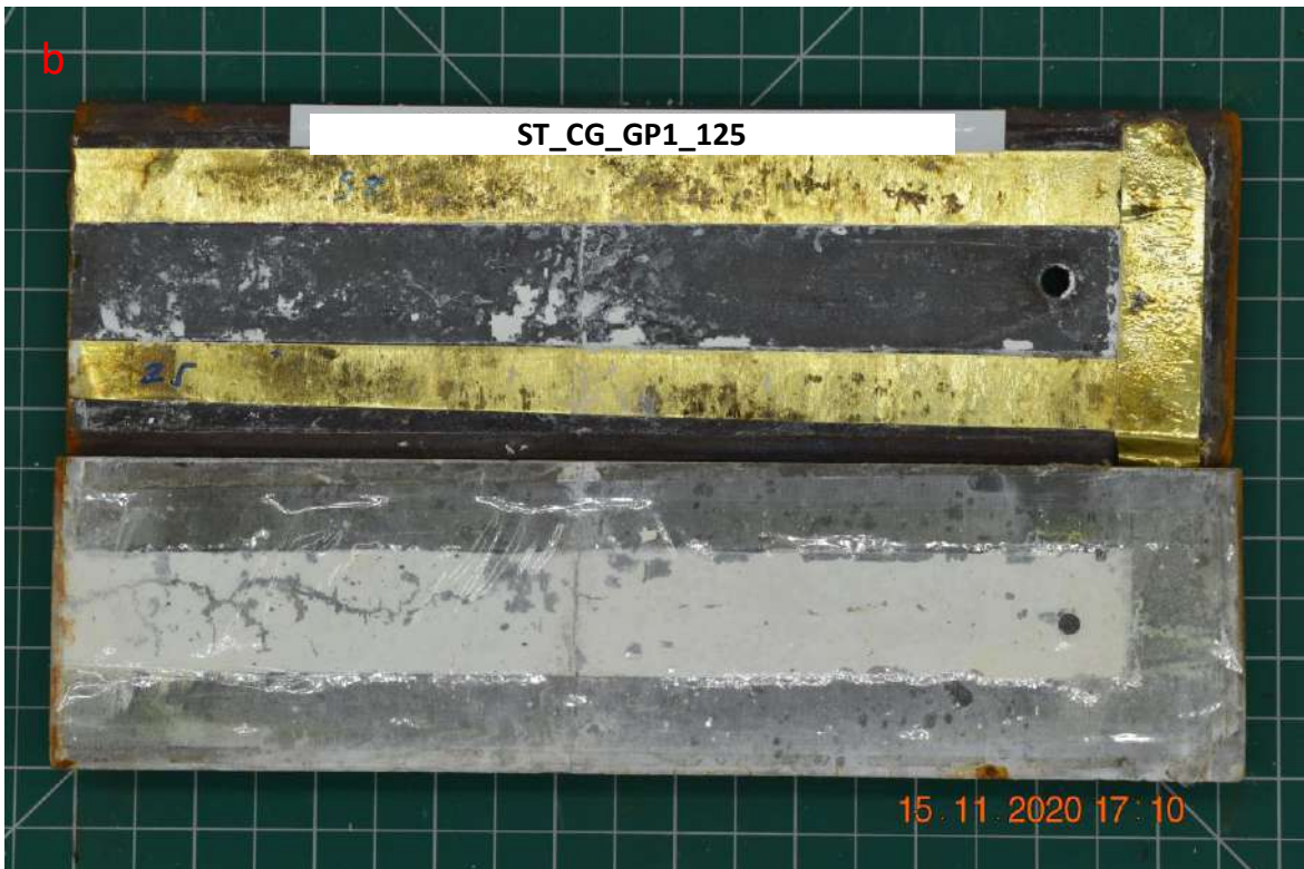
Figure C. 9. Injection test for fracture sample ST_CG_GP1_125, a) Injection pressure, rate, force and volume vs time, and b) Photo of tested sample.
