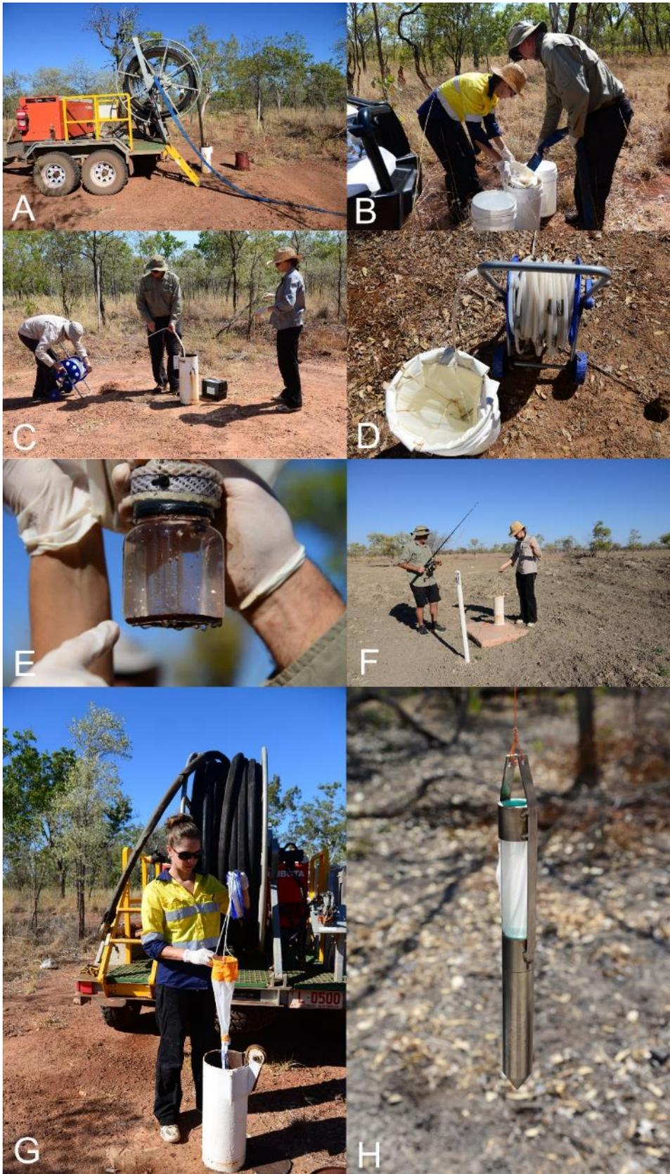
Figure 4. Range of sampling methods used; A: large motorised pump; B: filtering pumped water through large plankton net; C: small motorised pump; D: filtering pumped water through large plankton net using small pump; E: catching jar; F: lowering nets down bore hole using fishing rod; G: lowering medium-sized plankton net down bore hole using manual fishing reel; H: custom-made small-sized plankton net.
