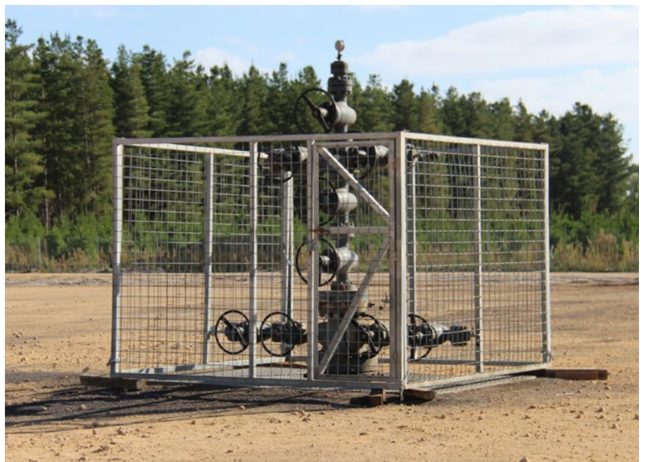
The Haselegrove 3 conventional gas exploration well head adjacent to commercial pine forestry operations near Penola
