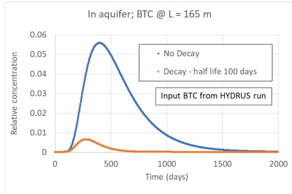
Breakthrough curve for receptor located @ 165 m due to input shown in Figure 1; for half life = 10 days,  $C \approx 3 \times 10^{-7}$
