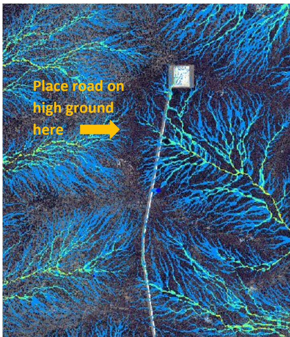
Figure 5 Map of a woodland area after gas development and surface water flows demonstrating the areas of highest erosion risk. This example shows how careful placement of infrastructure can allow for water to flow away from roads or pipelines, rather than across and along them. This image also suggests that a minor change in the placement of the access track could have further minimized potential risks.
