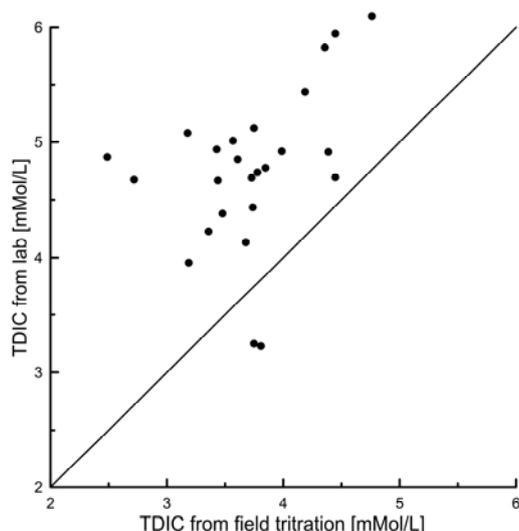
Figure 3.3 Comparison between field titration and laboratory analysis for Total Dissolved Inorganic Carbon (TDIC).
