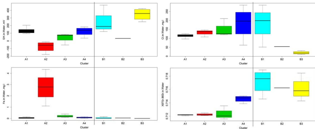
Figure 4.6 Boxplots with median and range for Eh, pH, Fe concentration, and  $^{87}\text{Sr}/^{86}\text{Sr}$  ratio for the calculated clusters. Outliers are presented as small circles.
