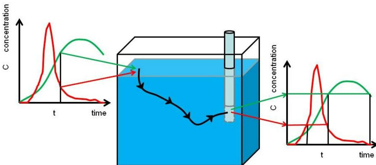
**Figure A.1: Principle of the application of environmental tracers to deduce groundwater age (Suckow 2014a)**
