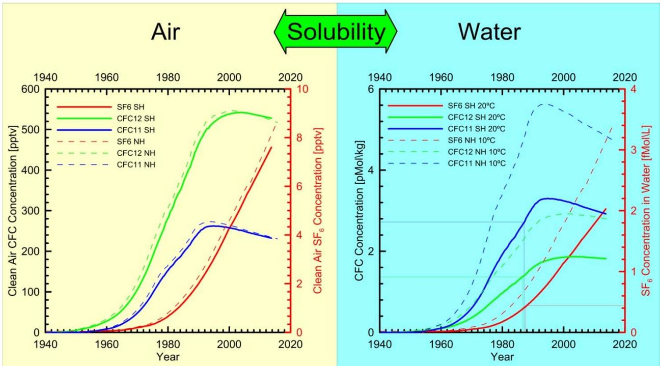
**Figure A.3: The principle how CFCs and SF<sub>6</sub> are used to deduce time, SH and NH being ‘southern’ and ‘northern’ hemisphere respectively**
