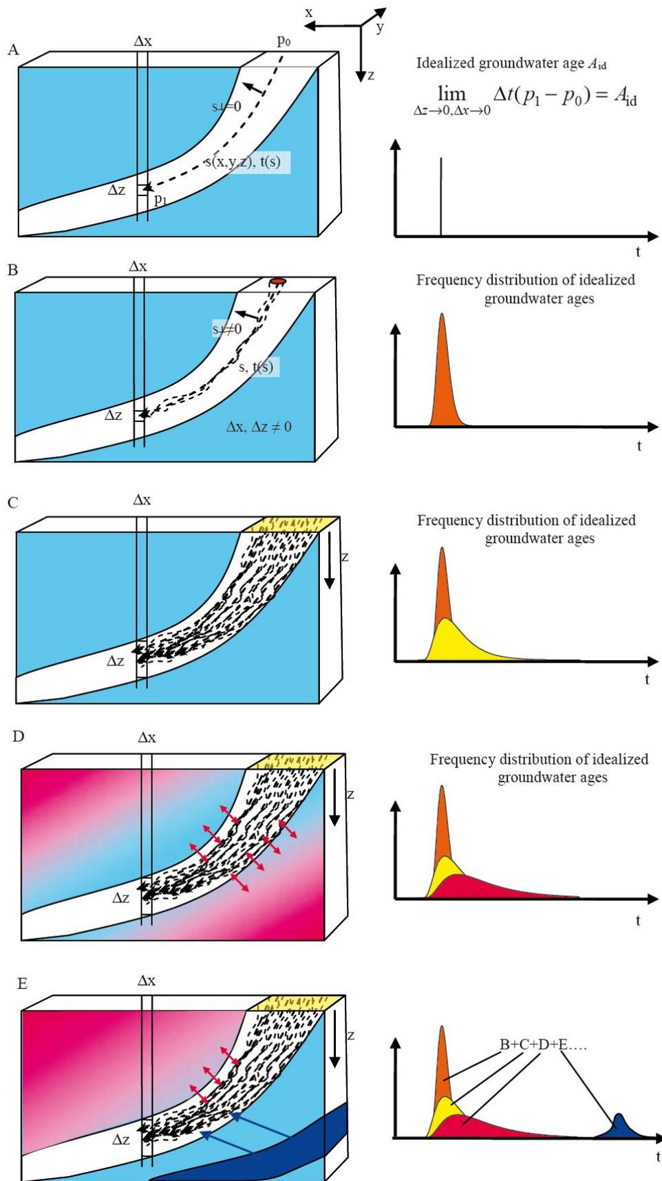
**Figure A.9: Spreading of age distributions due to different processes relevant in groundwater (Torgersen et al. 2013)**
