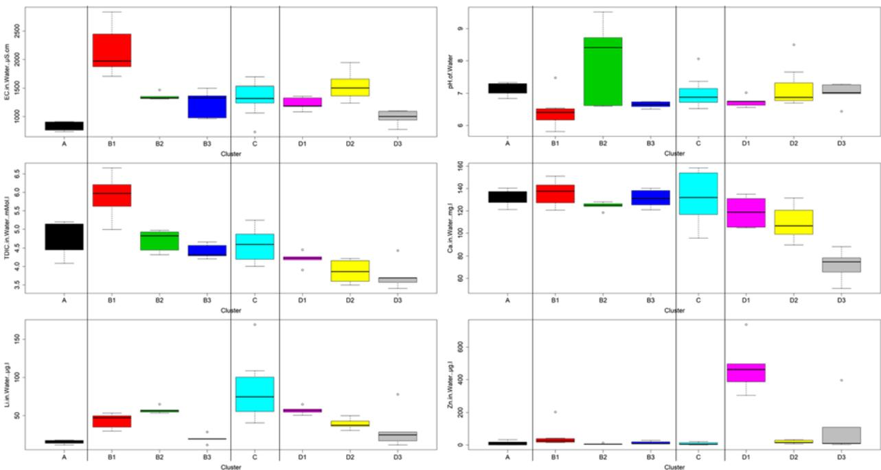
Figure 4.3 Boxplots of median and range of electrical conductivity (EC), pH, and concentrations for TDIC, Ca, Li, and Zn for the calculated clusters.
