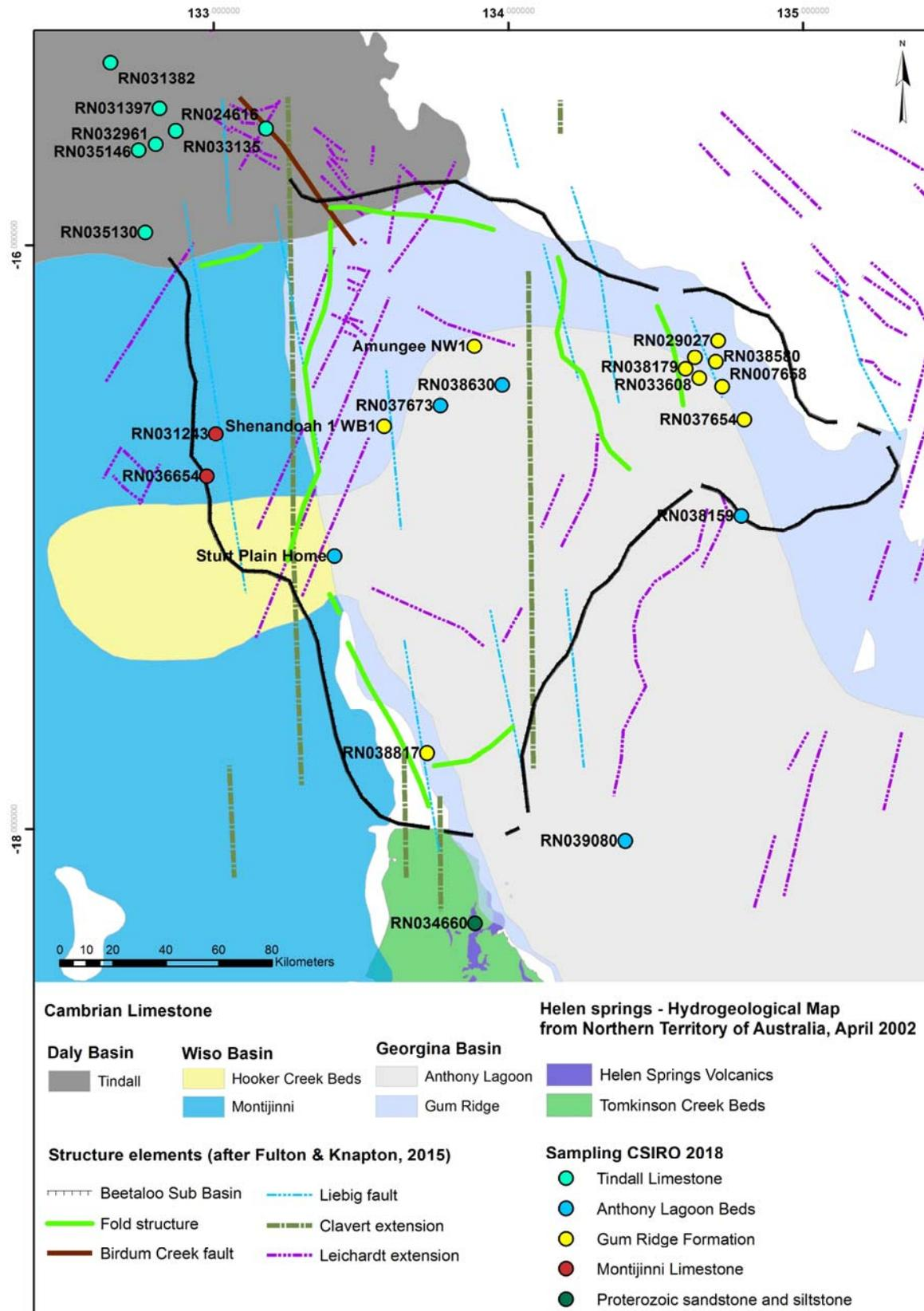
Figure 3.2 Hydrogeological map of the Beetaloo Sub Basin including the sampling locations
