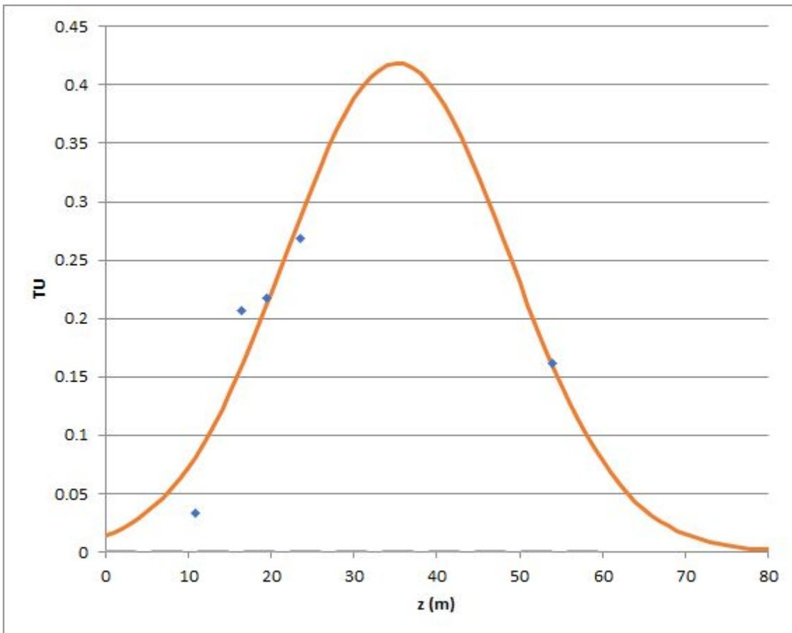
**Figure 5.4** Plot of a Gaussian profile fitted to integrate the measured tritium signals.  $z$  is the depth screen midpoint below water level, peak position is at 35 m below groundwater.
