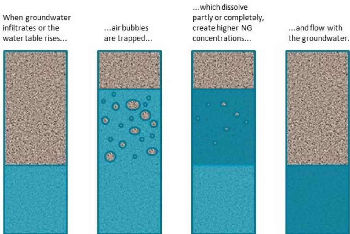
Figure A.8: The process of Excess Air formation.
