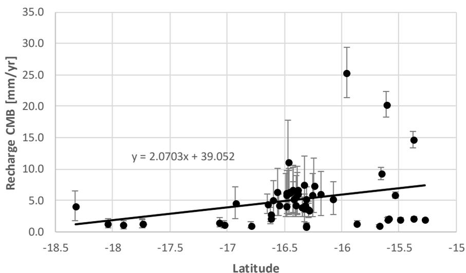
**Figure 5.2** Groundwater recharge estimated with the chloride mass balance method as a function of the latitude of the sampling locations.
