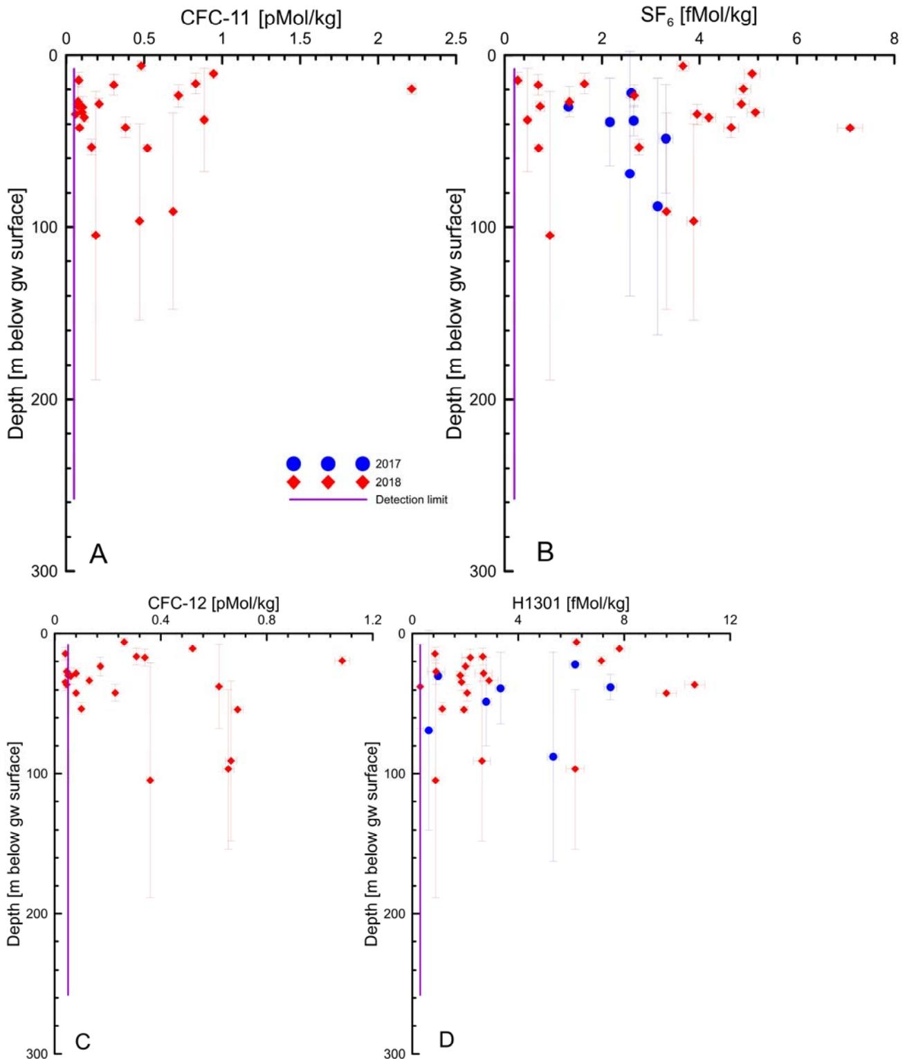
**Figure 4.10** Plot of concentration versus depth below water level for transient gas tracers
