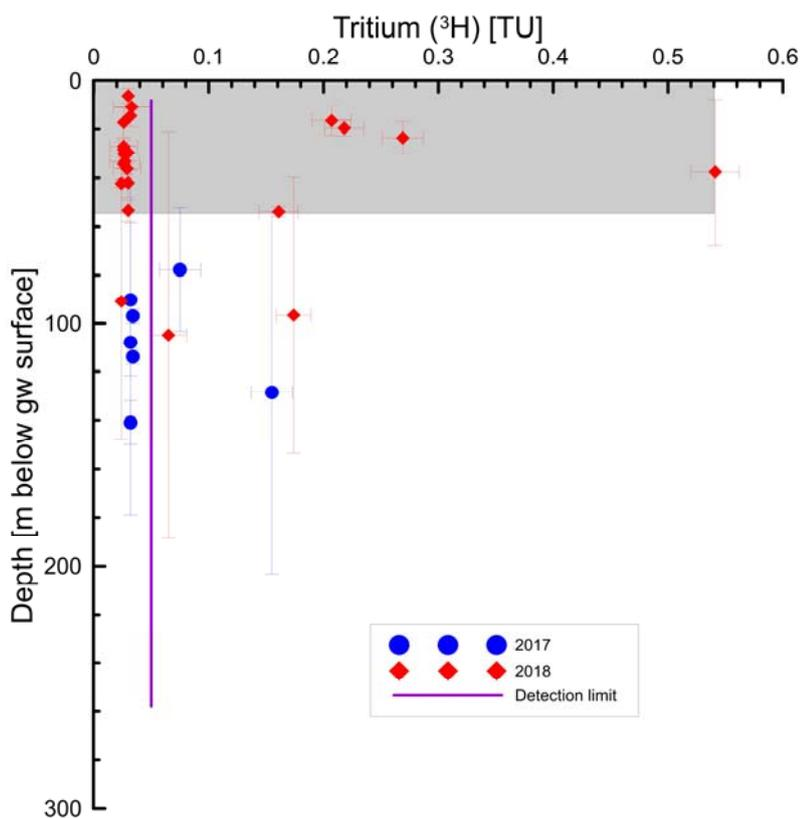
**Figure 4.8 Plot of measured tritium (TU) vs. screen depth below groundwater. Vertical error bars indicate the screen length. The shaded box represents the measurements used for recharge calculation (see discussion).**
