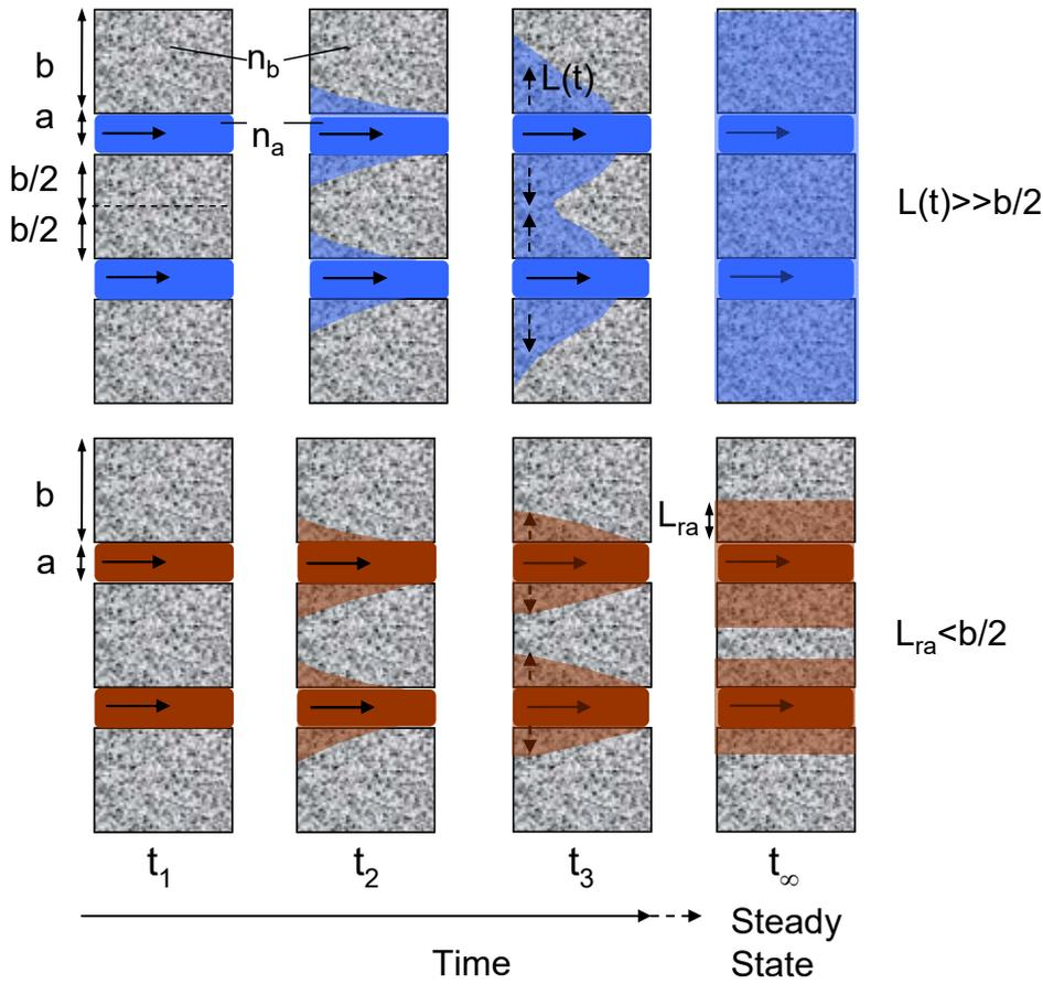
Figure A.10: Tracer retardation by matrix diffusive loss into stagnant zones (Purtschert *et al.* 2013)
