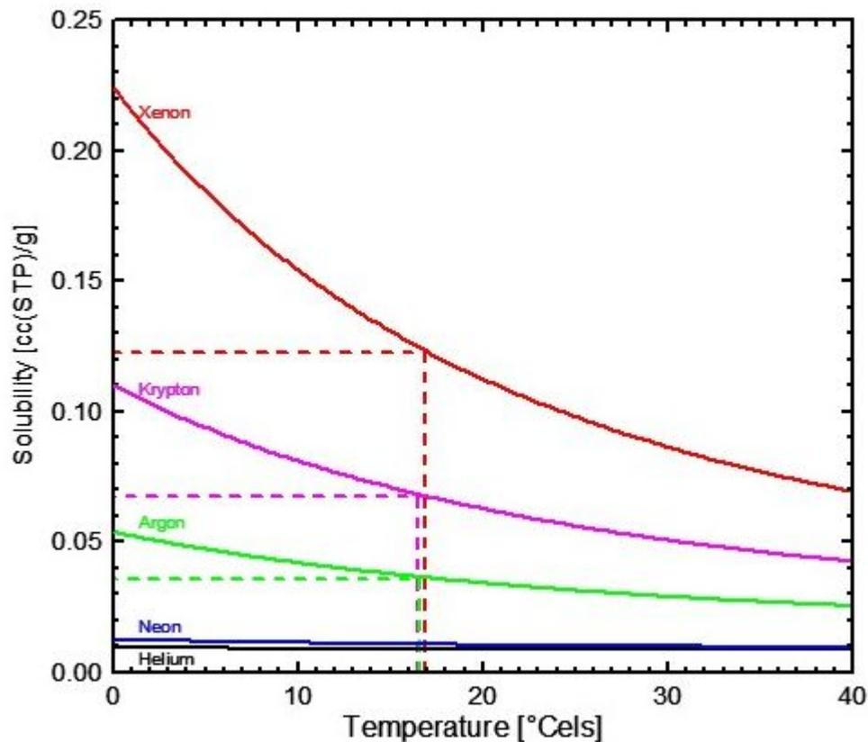
Figure A.7: Solubility of the noble gases as function of temperature in fresh water at sea level.
