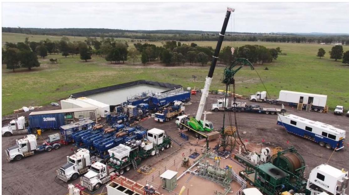
**Figure 1 Hydraulic fracturing of a well in the Surat Basin**
