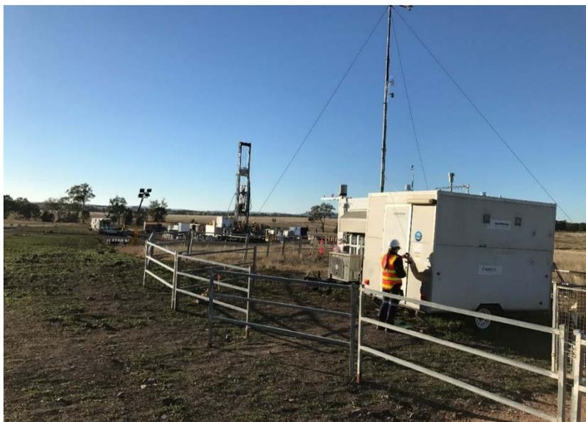
**Figure 7** Two enclosures at North-AQMS located adjacent to a well pad undergoing drilling.
