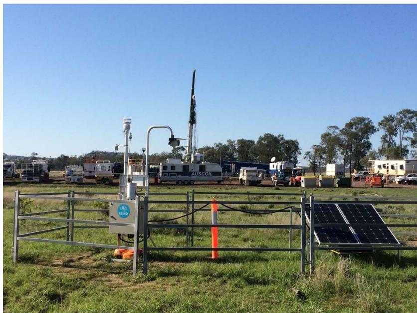
Figure 8 Solar-AQMS #4 located adjacent to a well pad (COM 314) undergoing well perforation.
