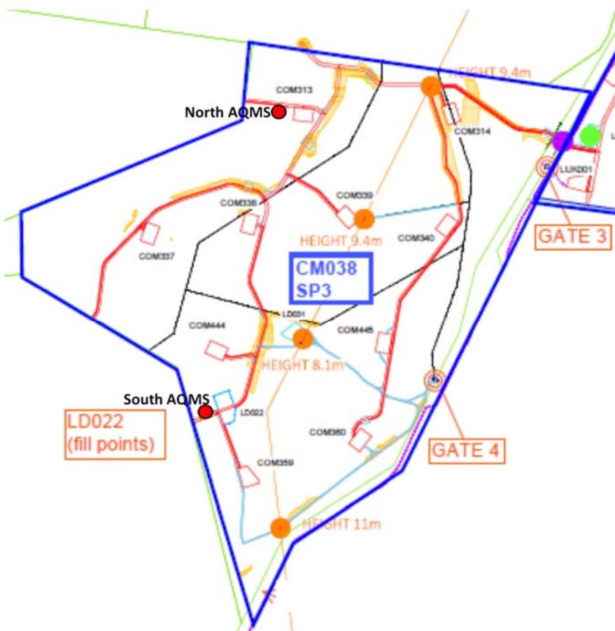
Figure 34 Map of HF study site with North and South-AQMS (red dots), roads, wells (COM###) and laydown area near South-AQMS shown. Source: Origin Energy.
