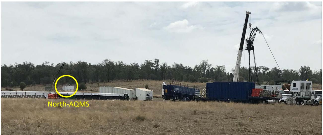
Figure 5 North-AQMS with HF spread present at adjacent well (COM 313) in the foreground. The distance from the COM 313 to the North-AQMS was approximately 100 m.
