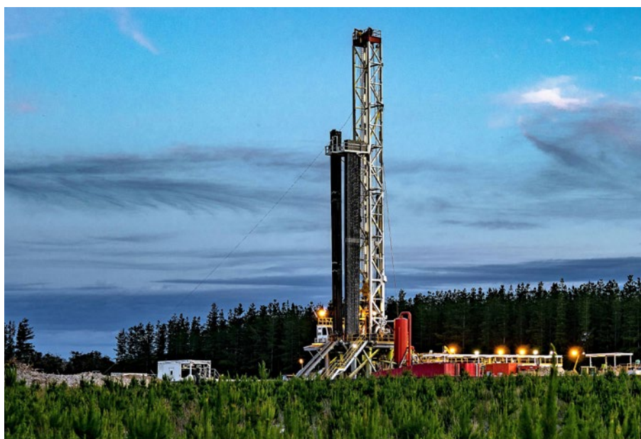
Conventional gas exploration drill rig operating in south east South Australia.
