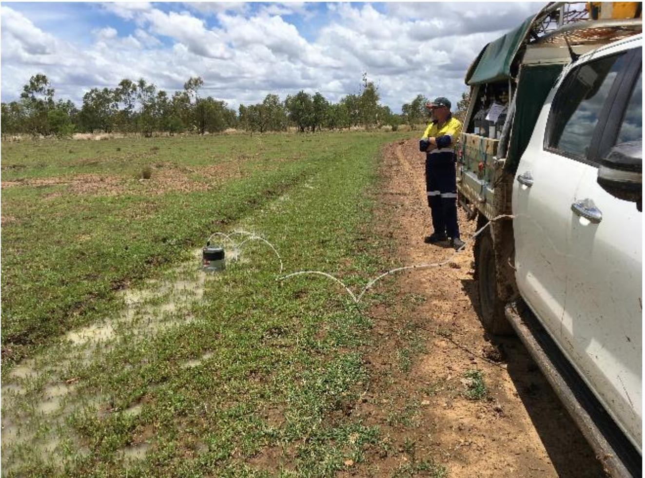
Figure 5: Surface flux chamber used for measuring soil CH<sub>4</sub> emissions. This chamber was also used for measuring CH<sub>4</sub> emissions from some termite mounds. The particular measurement was taken on saturated soils.
