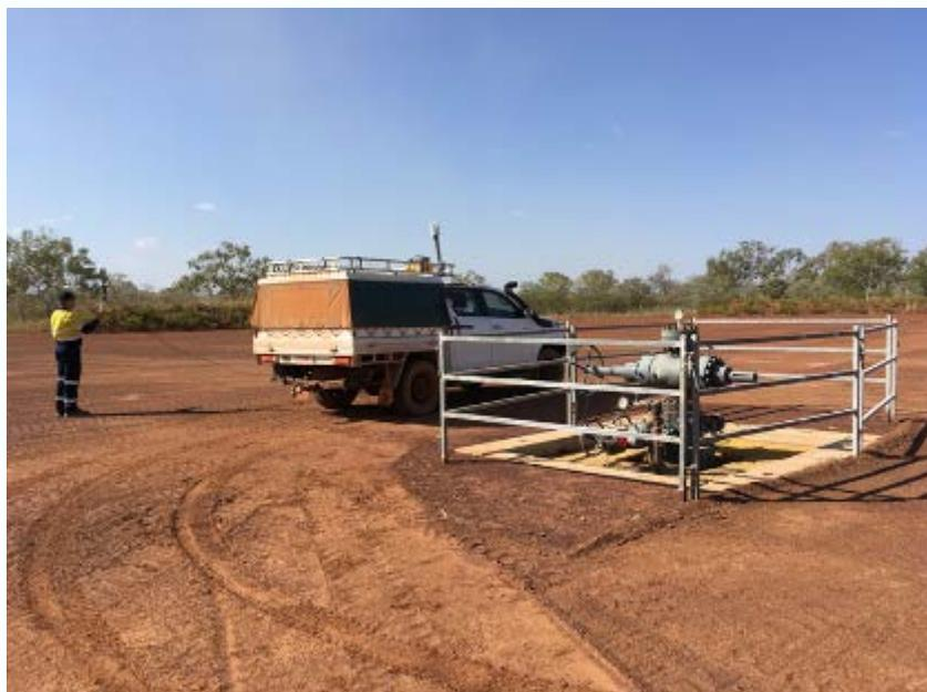
Figure 14: Collecting CH<sub>4</sub> and wind measurements at the West Beetaloo 1 suspended well.
