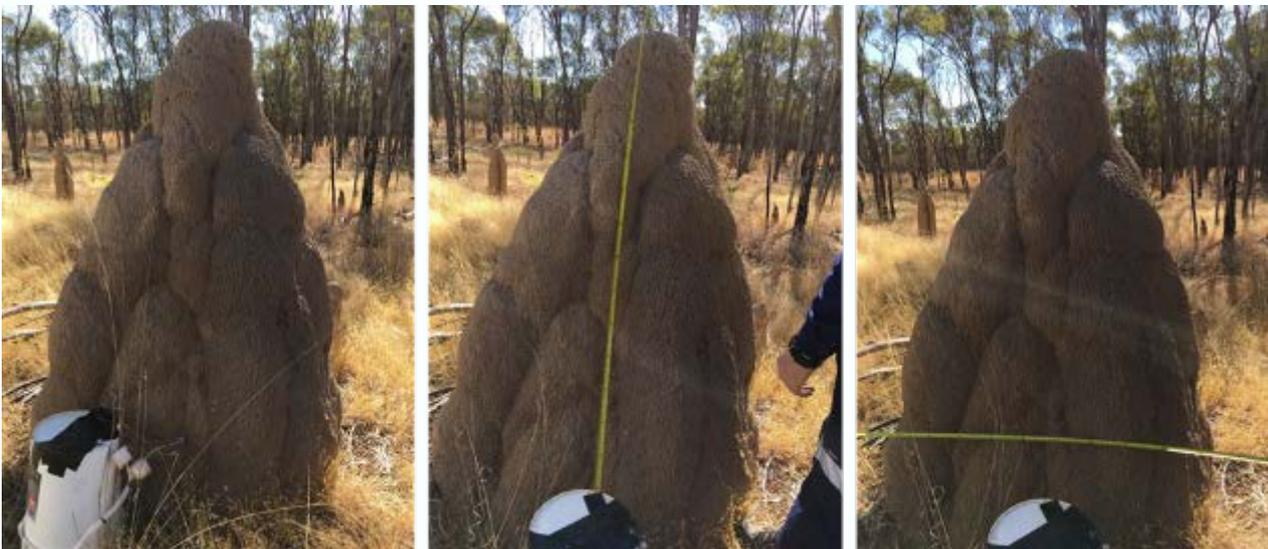
Figure 29: Large termite mound measured at the side with a 20-litre flux chamber (middle photo) and with the tubing inserted into the side of the mound (left photo).
