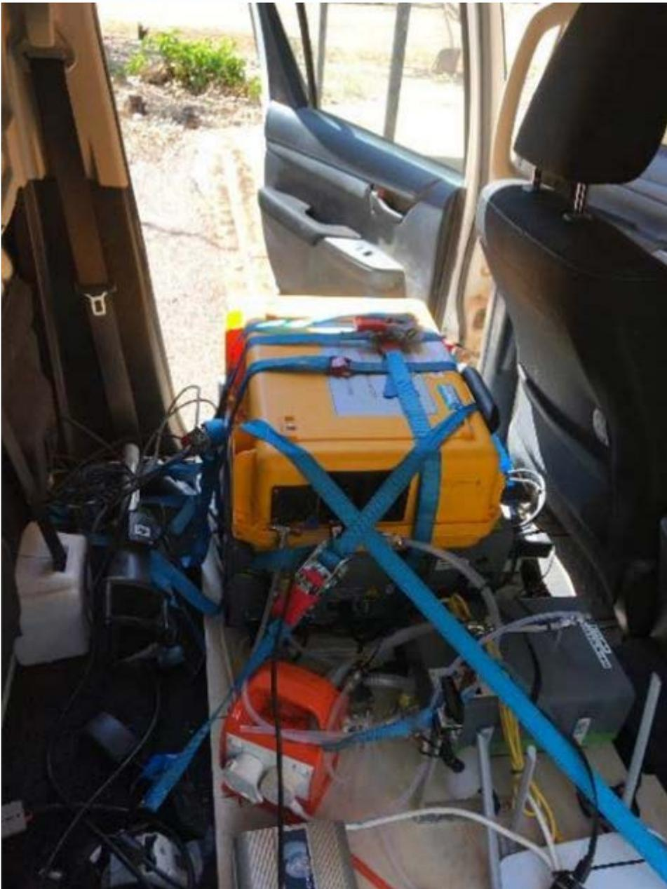
Figure 4: PICARRO and LGR analysers mounted in the back seat of the field vehicle. Note that the back seat has been removed.
