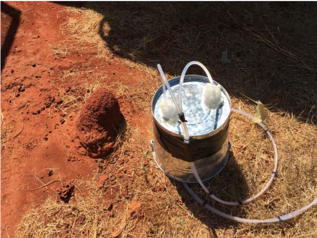
Figure 28: Small termite mound measured with a 9-litre flux chamber.
