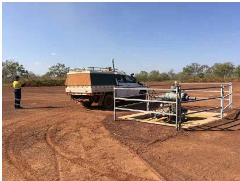
Figure 12: Collecting CH 4 and wind measurements at the West Beetaloo 1 suspended well.
