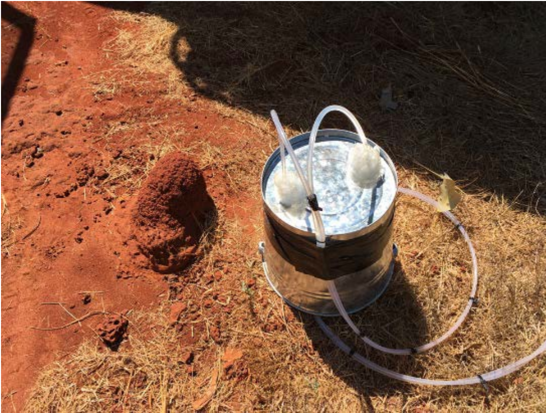
Figure 16: Small termite mound measured with a 9-litre flux chamber.
