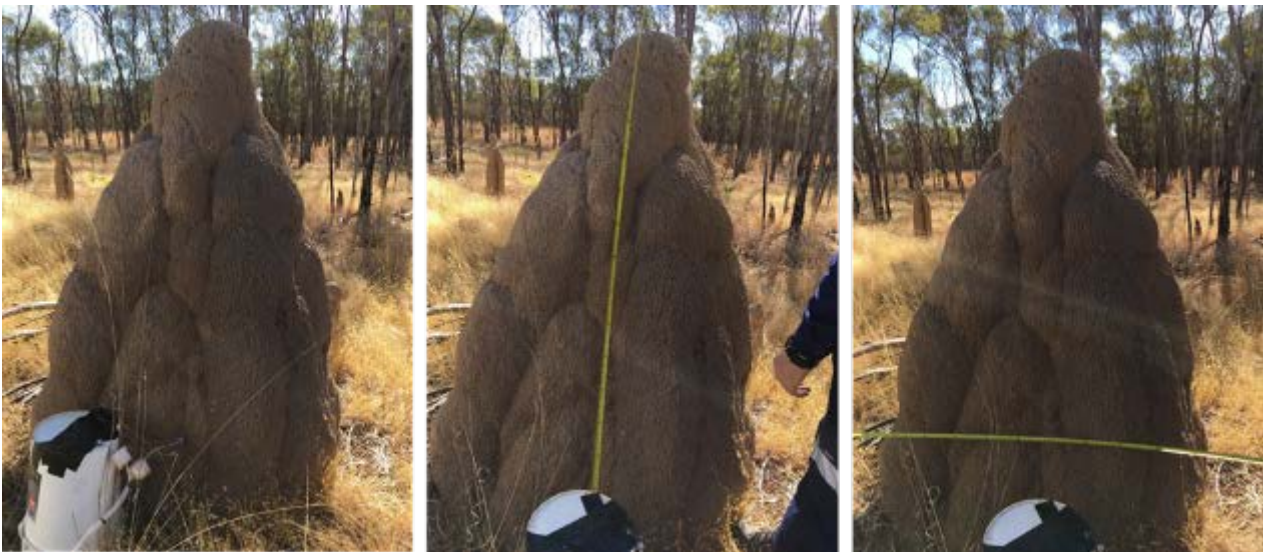
Figure 17: Large termite mound measured at the side with a 20-litre flux chamber (middle photo) and with the tubing inserted into the side of the mound (left photo).
