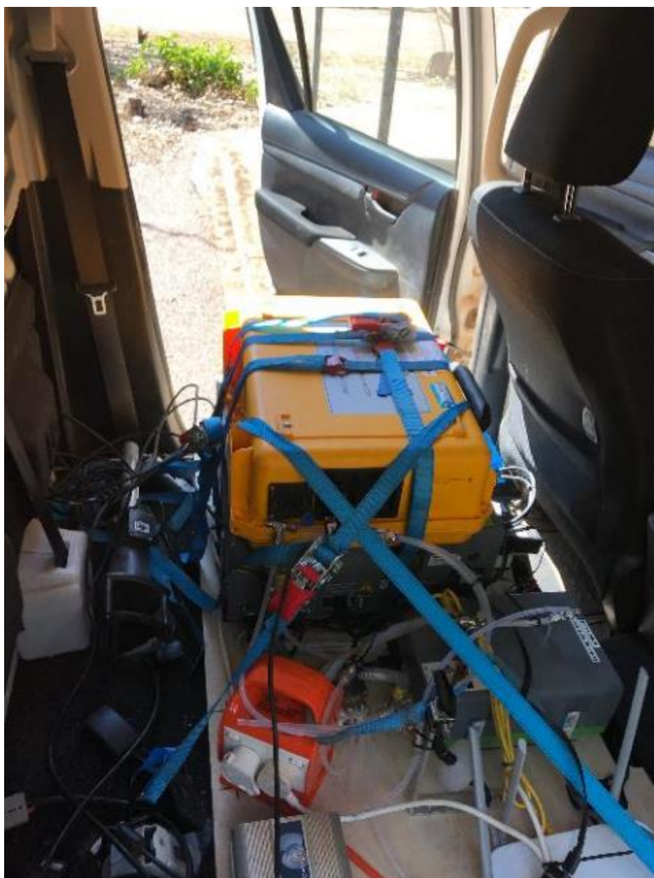
Figure 2: PICARRO and LGR analysers mounted in the rear of the field vehicle. Note that the back seat has been removed.
