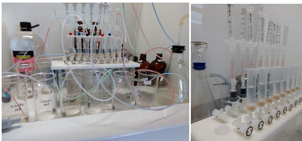
Figure 16. Views of the SPE apparatus set up at Reedy Creek
