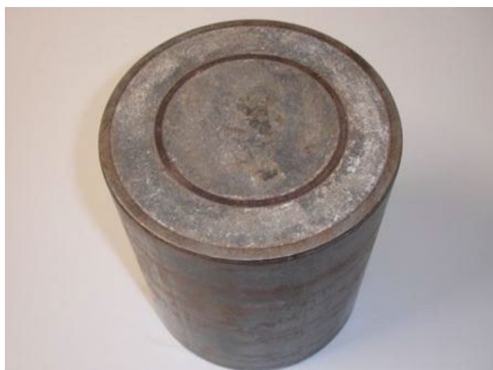
An example of casing and cement used in a decommissioned well.
