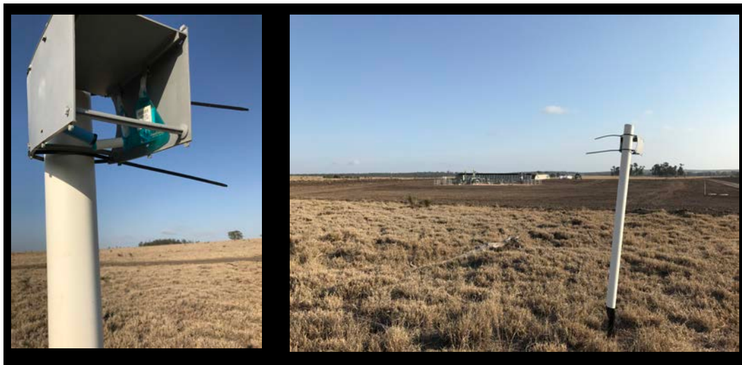
Figure 3 Passive Radiello samplers deployed in the field housed in weather proof covers and mounted on ~ 2m high poles.
