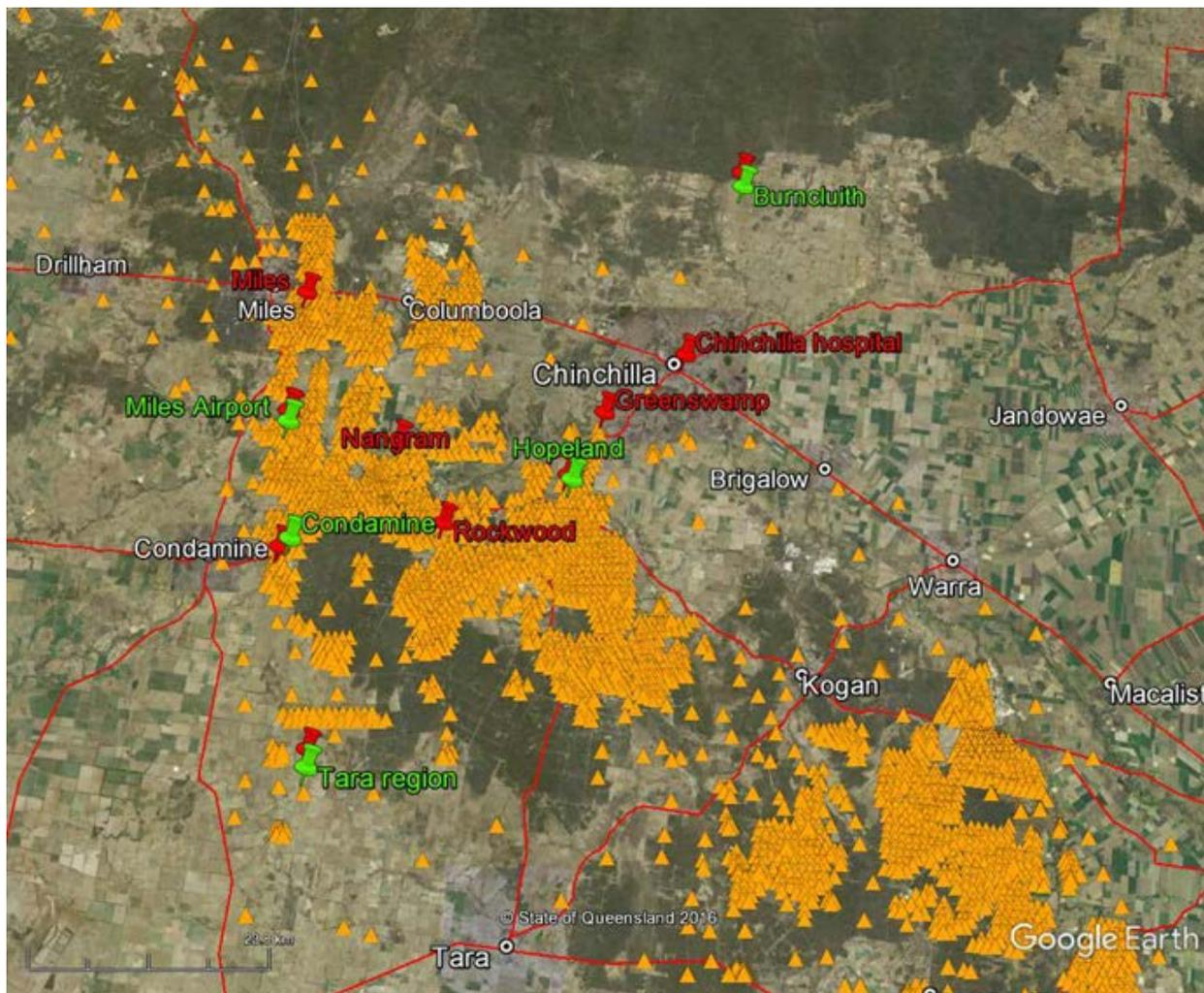
Map of project study area (town names in white text, green pins are ambient air monitoring sites, red pins are passive gas sites, orange triangles are CSG wells)
