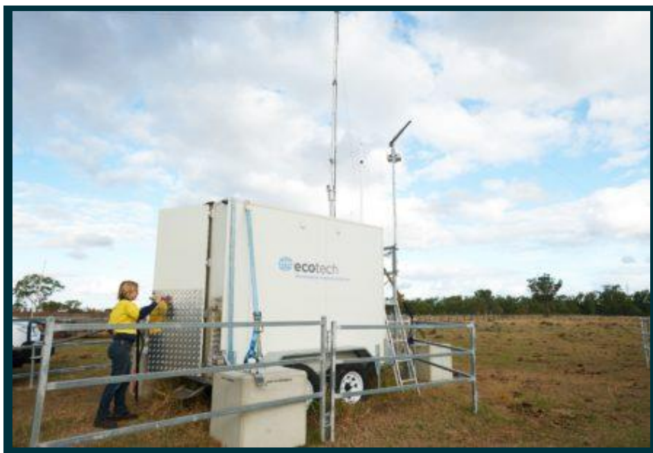
Figure 5 Mobile AQMS (Ecotech Australia). Two similar enclosures will be located at the AQMS site for the HF Study.
