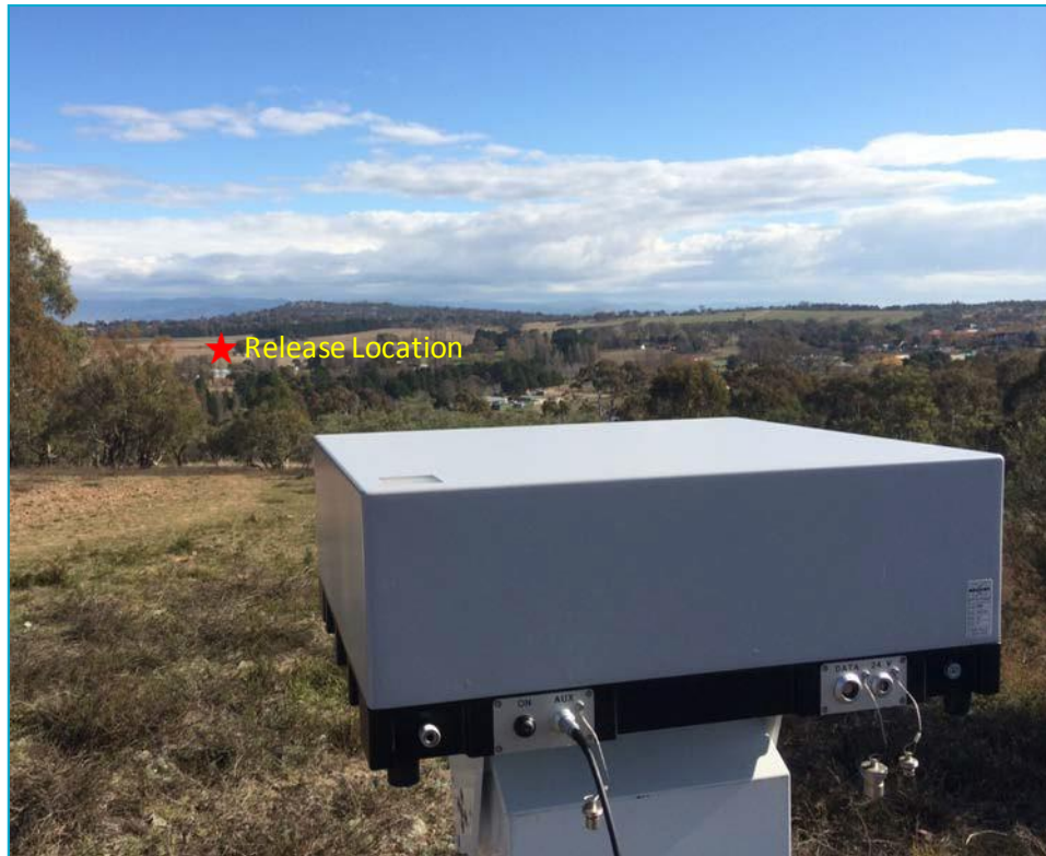
Figure 5.2. Bruker HI90 capturing data from a hill 1.5km from the Ginninderra experiment.
