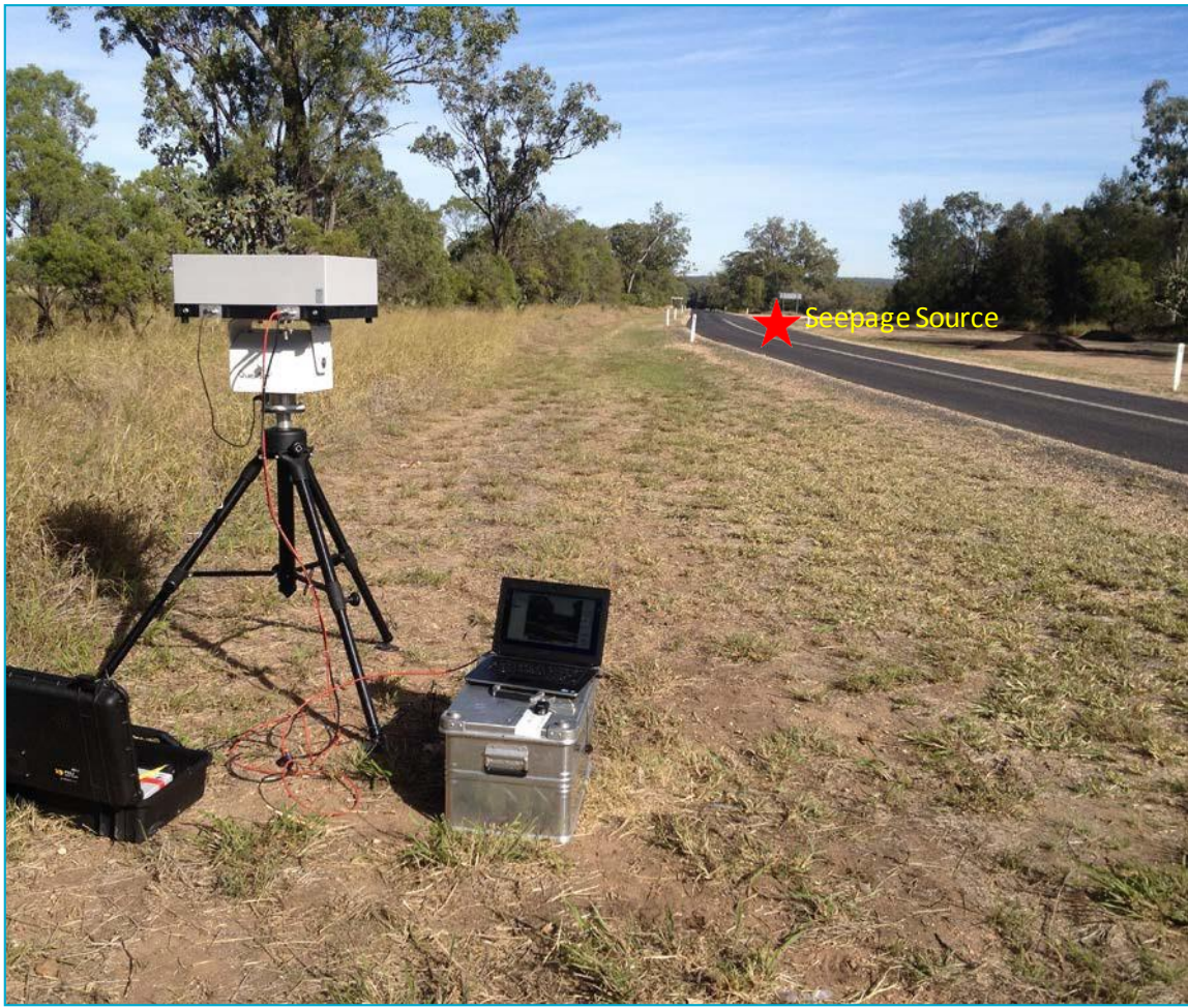
Figure 5.3. Bruker HI90 set up to measure approximately 200m from the seepage source.
