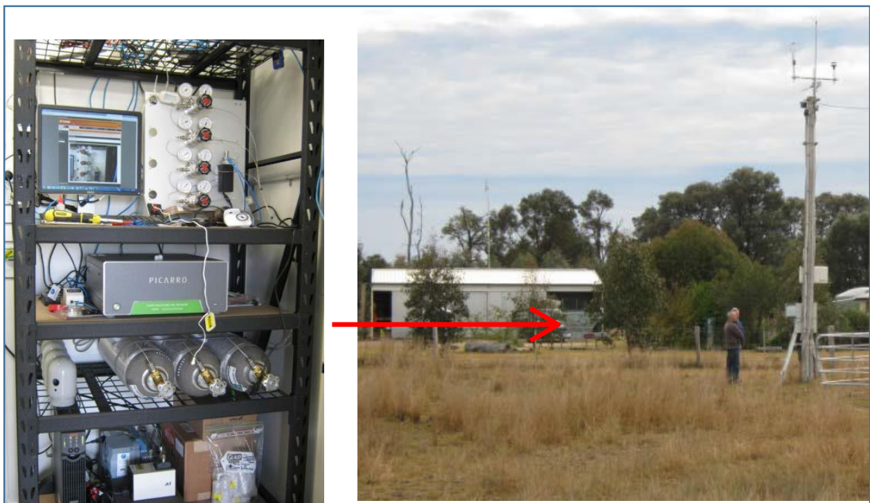
Figure 3.3. The Burncluth monitoring facility showing instruments and calibration gases (left) and the installed module and meteorological instruments on a nearby pole (right).
