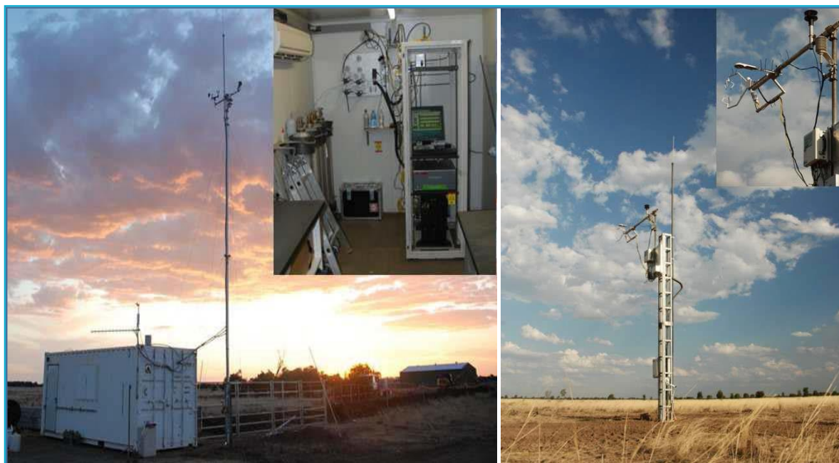
Figure 3.2. The Ironbark monitoring container (left) and concentration instruments (inset); the flux tower (right) and meteorological instruments (inset).
