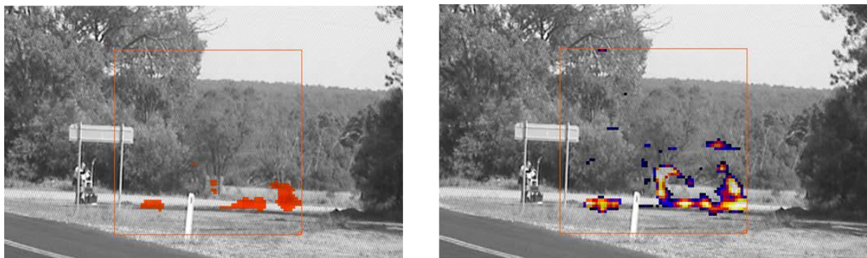
Figure 5.6.(a) Red shows areas where methane was detected at 200m from an old exploration bore near Chinchilla. (b) Relative abundances of methane. Colourscale is shown in Figure 5.
