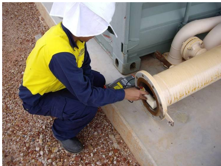
Figure 3: Contamination monitoring of spool – February 2010.
