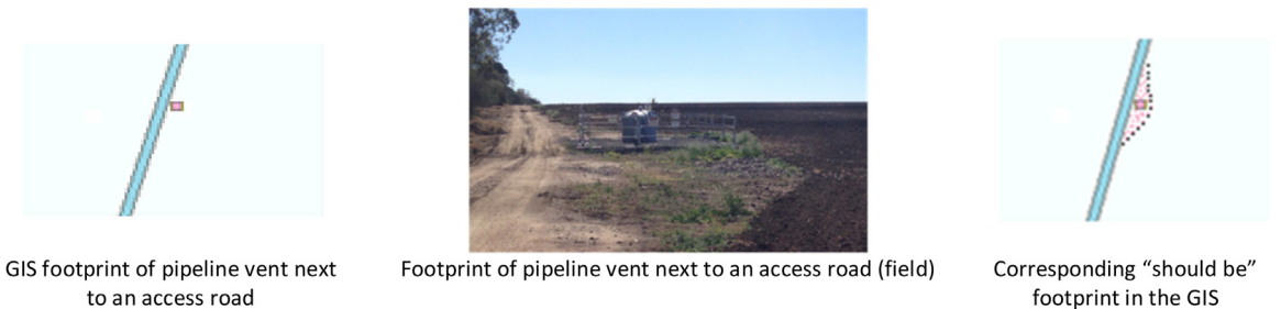
Fig. 7. Nominal footprint as shown in GIS (left). Observed footprint in the field (middle) and “should be” footprint in the GIS (right).
