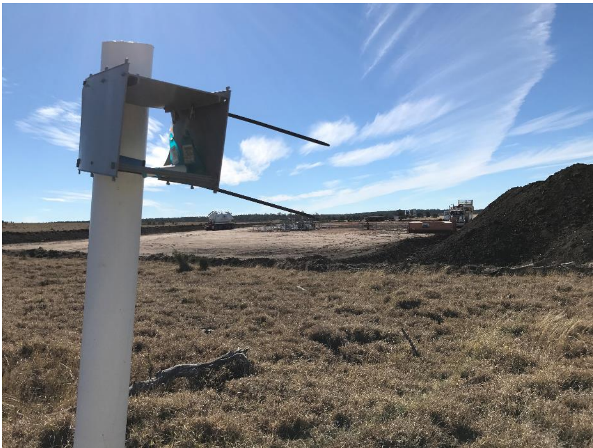
Figure 32 Radiello samplers deployed in the field
